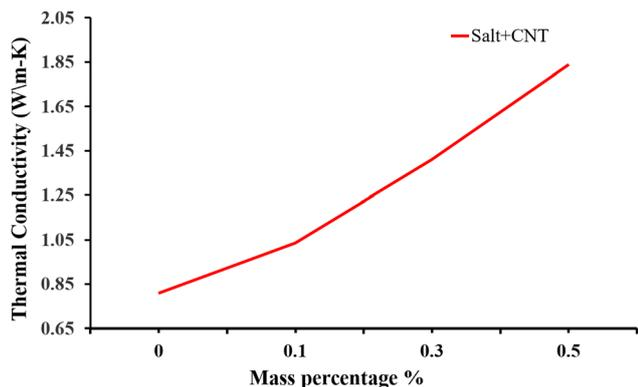
Fig. 22 Experimental data showing how the thermal conductivity of  $\text{NaNO}_3\text{-KNO}_3$  improves with addition of CNT at different mass concentrations of 0.1%, 0.3% and 0.5%. Adapted from ref. 39, with permission from the American Chemical Society, Copyright 2023.
