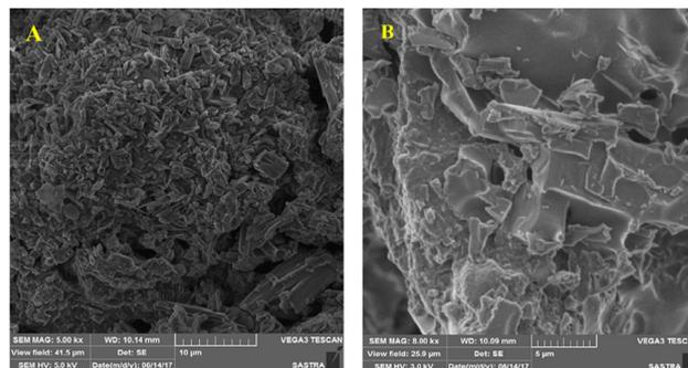
Fig. 21 SEM images of pure (A) and CNT-enhanced solar salt, and (B). Adapted from ref. 39, with permission from the American Chemical Society, Copyright 2023.
