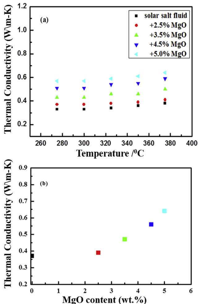
Fig. 20 Experimental data showing the thermal conductivity of  $\text{NaNO}_3\text{-KNO}_3$  (a) improves with the addition of MgO at different mass concentrations (2.5%, 3.5%, 4.5% and 5%) with temperature, and (b) the increasing thermal conductivity at different concentrations. Adapted from ref. 35, with permission from Elsevier, Copyright 2020.
