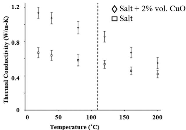
Fig. 18 Experimental data showing elevation in thermal conductivity before and after addition of CuO nanoparticles to  $\text{NaNO}_3\text{-KNO}_3$ . Adapted from ref. 34, with permission from Elsevier, Copyright 2016.
