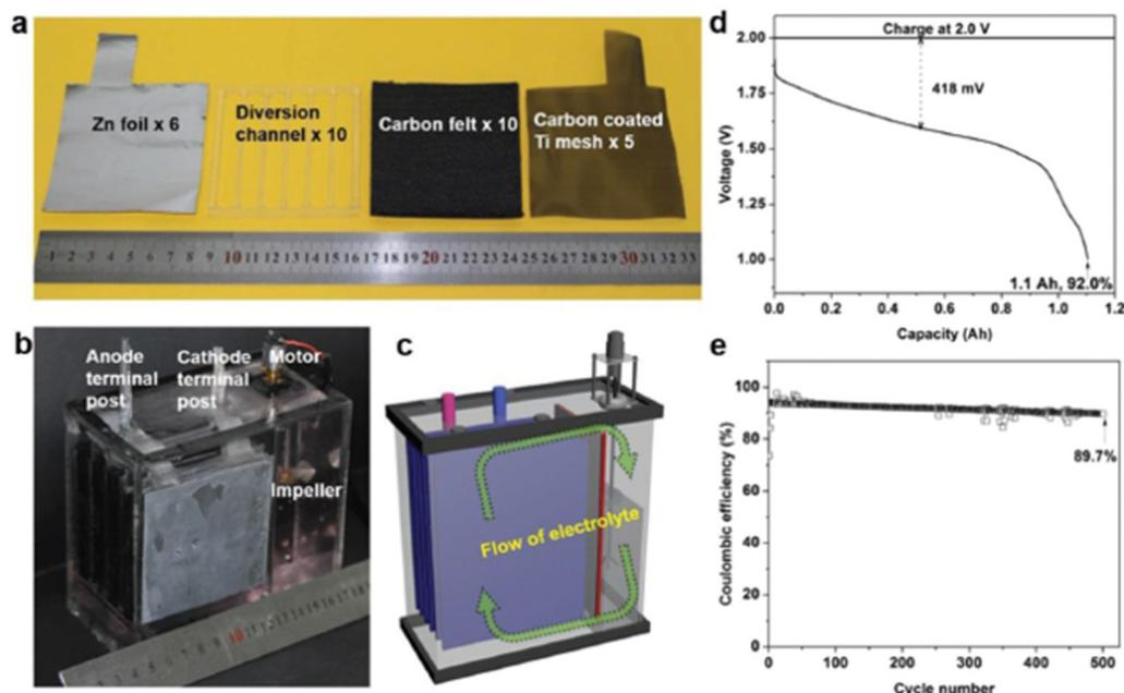
Fig. 15 (a) The cell components used for the membrane free aqueous Zn/MnO<sub>2</sub> RFB, (b) photographic image of the Zn/MnO<sub>2</sub> RFB, (c) schematic diagram of the indication of electrolyte flow, (d) the GCD profile of the Zn/MnO<sub>2</sub> RFB, and (e) the cyclability of the Zn/MnO<sub>2</sub> RFB (reproduced from ref. 87 with permission from Wiley).
