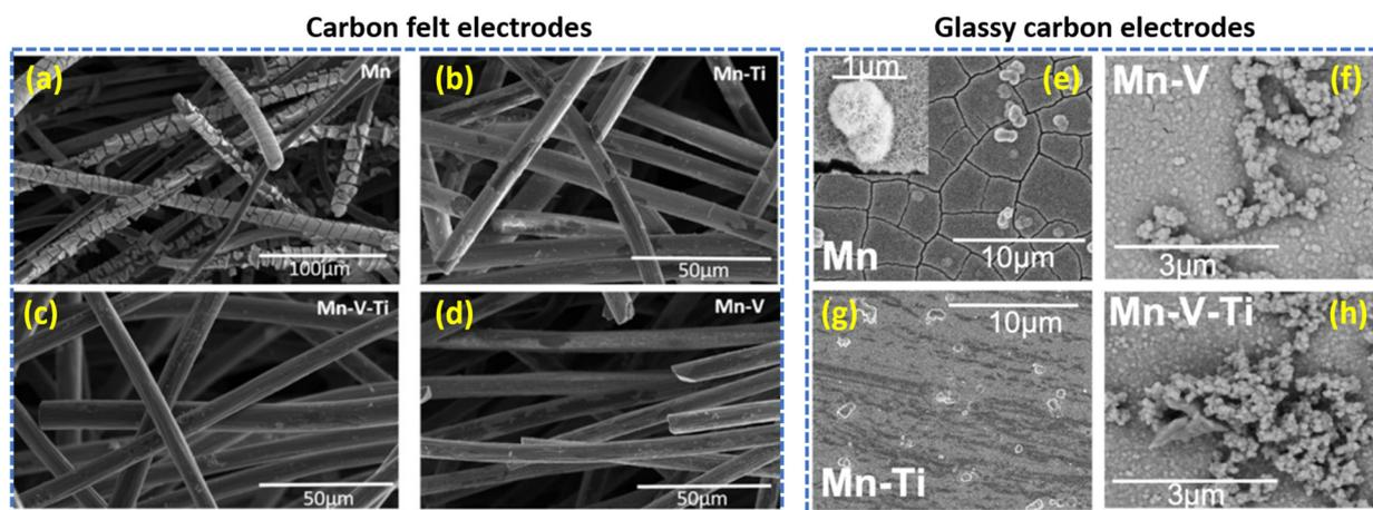
Fig. 11 SEM images of electrodeposited  $\text{MnO}_2$  on the carbon felt electrodes (a)–(d) and on the glassy carbon electrodes (e)–(h), respectively (reproduced from ref. 74 with permission from Wiley-VCH).
