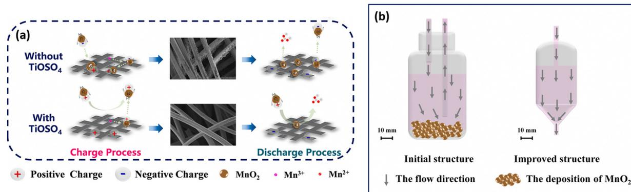
Fig. 6 Schematic illustration of (a) the TiOSO<sub>4</sub> additive in the V–Mn flow battery and (b) the improved electrolyte tank structure (reproduced from ref. 46 with permission from Elsevier).
