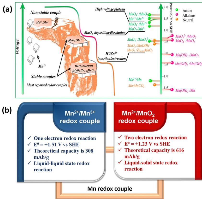
Fig. 4 (a) Schematic illustration of manganese redox couples in different electrolytes (reproduced from ref. 43 with permission from the American Chemical Society) and (b) comparison of  $Mn^{2+}/Mn^{3+}$  and  $Mn^{2+}/MnO_2$  redox couple characteristics.
