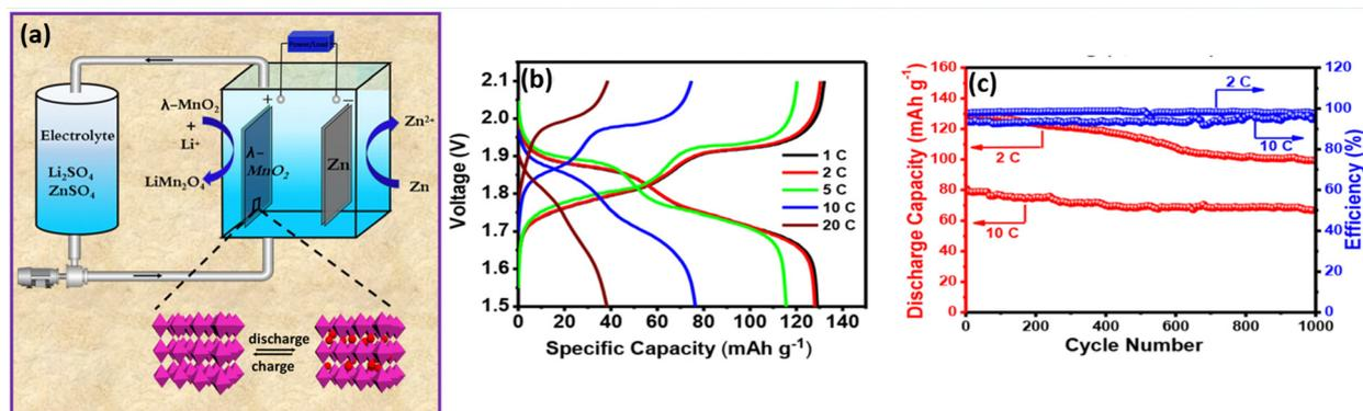
Fig. 14 (a) Schematic illustration of the single flow Zn/ $\lambda\text{-MnO}_2$  RFB, (b) the GCD profile of single flow Zn/ $\lambda\text{-MnO}_2$  RFB at different C rates, and (c) long cycling performance of Zn/ $\lambda\text{-MnO}_2$  RFB recorded at 2 and  $10\text{C}$  rates.<sup>86</sup>
