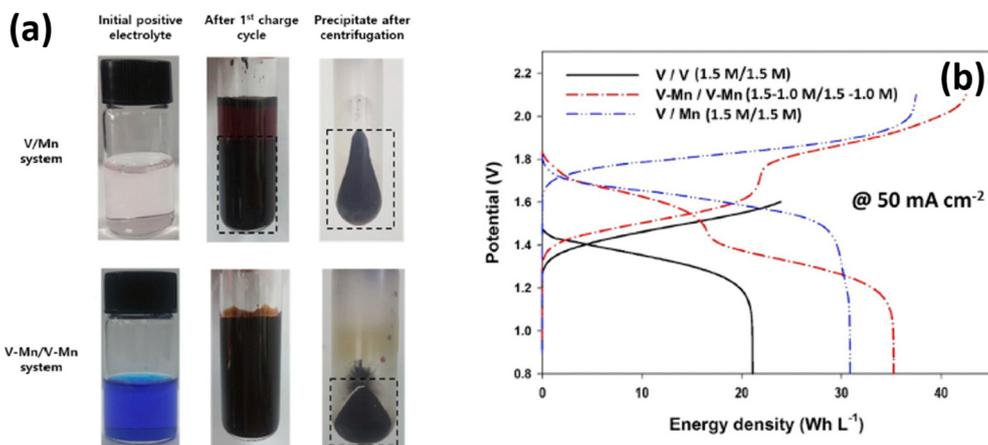
Fig. 10 (a) Photographic images of MnO<sub>2</sub> deposition in the V/Mn and V–Mn/V–Mn system and (b) GCD profile recorded at 50 mA cm<sup>-2</sup> (reproduced from ref. 72 with permission from Elsevier).
