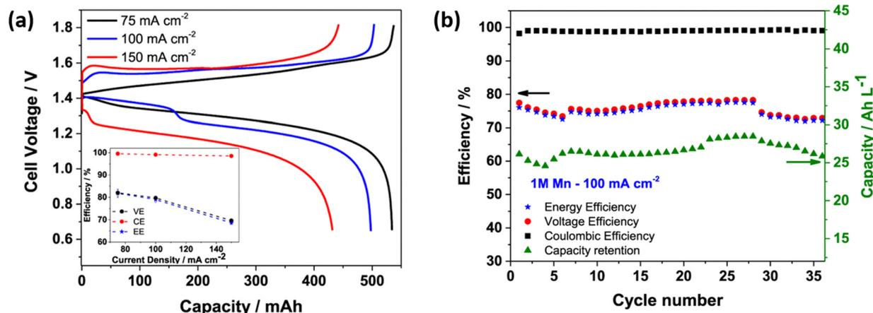
Fig. 7 (a) Galvanic charge discharge performance recorded at different current densities, and (b) H-Mn flow battery performance at  $100 \text{ mA cm}^{-2}$ ; electrolyte:  $1 \text{ M MnSO}_4 + 3 \text{ M H}_2\text{SO}_4 + 1 \text{ M Ti}(\text{SO}_4)_2$ , Hydrogen:  $100 \text{ mL min}^{-1}$ , Flow rate:  $50 \text{ mL min}^{-1}$ , respectively.<sup>55</sup>
