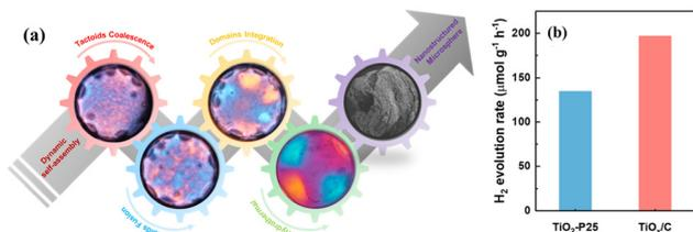
Fig. 11 (a) Schematic illustration of the synthesis and (b) the H<sub>2</sub> generation of TiO<sub>x</sub>/C microspheres with chiral nematic structures. Reprinted with permission from ref. 109. Copyright © 2021, American Chemical Society.
