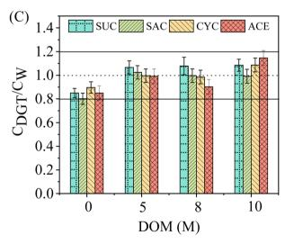
Fig. 3 Effects of pH (A), ionic strength (B), and DOM (C) on the ratios of ASs concentrations measured by WAX-XDA1-DGT devices to the solution concentrations ( $C_{\rm DGT}/C_{\rm W}$ ). The dotted horizontal lines represent the values at 1 and the solid horizontal lines represent the values at 0.8 and 1.2. Error bars: 1 SD (n = 3). SUC: Sucralose, SAC: Saccharin, CYC: Cyclamate, ACE: Acesulfame, DOM: dissolved organic matters.
