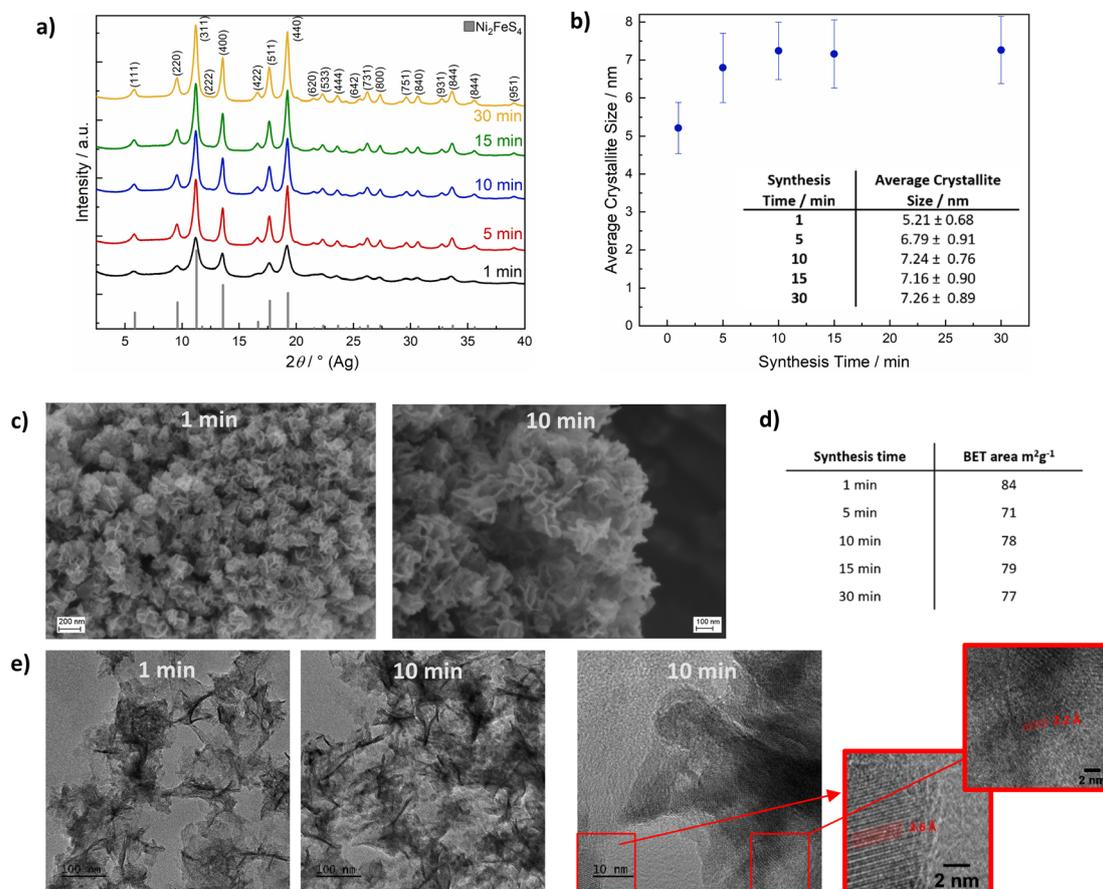
Fig. 2 XRD patterns for  $\text{Ni}_2\text{FeS}_4$  obtained after different synthesis times (a), corresponding crystallite sizes as determined by the integral breadth method (b), SEM images of  $\text{Ni}_2\text{FeS}_4$  nanosheets obtained after 1 and 10 min (c) and BET surface areas (d). For the identification of reflections, the ICDD reference card 00-047-1740. Additionally, TEM images of  $\text{Ni}_2\text{FeS}_4$  nanosheets obtained after 1 and 10 min are shown in (e).
