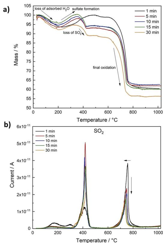
Fig. 4 Relative mass loss during TG-MS measurements in air for Ni<sub>2</sub>FeS<sub>4</sub> obtained after different synthesis durations (a) and SO<sub>2</sub> evolution detected by MS depending on the temperature (b).
