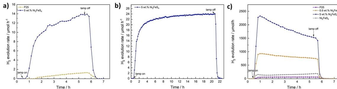
Fig. 8 Photocatalytic HER over P25 and 5 wt% Ni<sub>2</sub>FeS<sub>4</sub>@P25 using ethanol as a scavenger (a), for longtime irradiation (1 sun) of 5 wt% Ni<sub>2</sub>FeS<sub>4</sub>@P25 in aqueous methanol solutions (b), as well as HER rates under UV irradiation (c).
