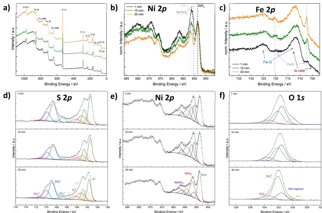
Fig. 3 XPS spectra for  $\text{Ni}_2\text{FeS}_4$  obtained after different synthesis durations. Survey scan (a), Ni 2p spectra normalised to the Ni–S peak for qualitative comparison (b), normalised Fe 2p spectra (c), as well as fitted S 2p (d), Ni 2p (e) and O 1s spectra (f).
