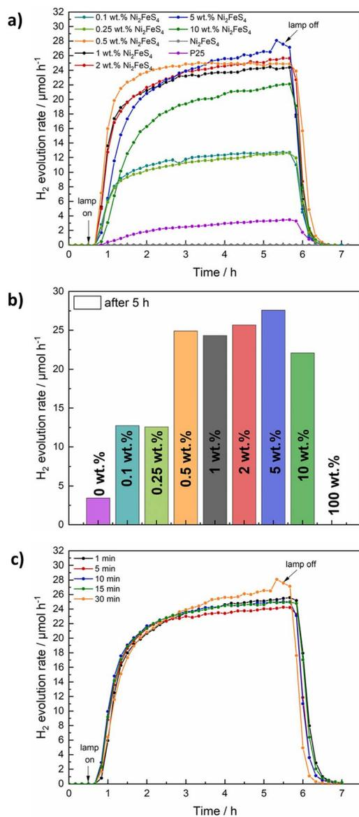
Fig. 6  $\text{H}_2$  evolution over P25 loaded with different amounts of  $\text{Ni}_2\text{FeS}_4$  under 1 sun simulated sunlight (a and b). Additionally, the  $\text{H}_2$  evolution for 5 wt%  $\text{Ni}_2\text{FeS}_4$ @P25, with  $\text{Ni}_2\text{FeS}_4$  obtained after different synthesis durations in the microwave is shown (c). The lamp was switched on after 30 min and turned off after 5 h of irradiation.
