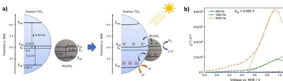
Fig. 7 Band positions of TiO<sub>2</sub> and Ni<sub>2</sub>FeS<sub>4</sub> before and after contact (a) and Mott–Schottky plots for Ni<sub>2</sub>FeS<sub>4</sub> in 0.5 M Na<sub>2</sub>SO<sub>4</sub> (values are already converted to pH 0) (b).
