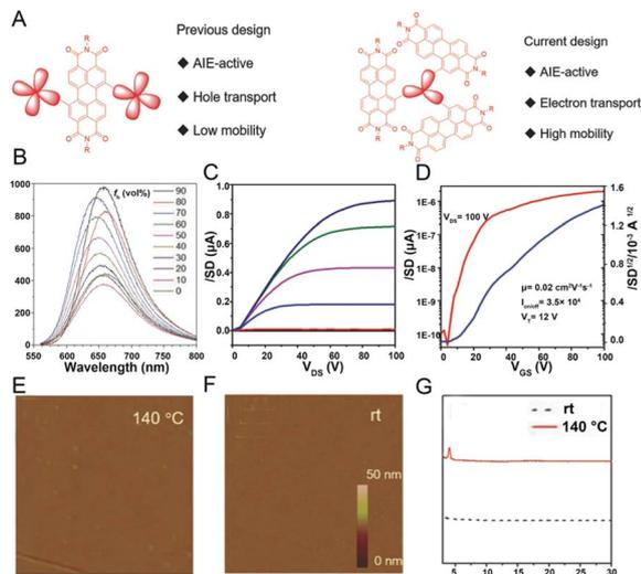
Fig. 16 (A) The design principles of AIEgen-based OFET devices. (B) TriPE-3PDI in CHCl<sub>3</sub>/hexane mixtures with different hexane fractions ( $f_h$ ). (C) Transfer and (D) output characteristics for OTFT devices of TriPE-3PDI annealed at 140 °C. AFM images of TriPE-3PD at (E) 140 °C and (F) at room temperature. (G) XRD patterns of thin films of TriPE-3PDIL at room temperature and 140 °C. Reproduced with permission from ref. 176. Copyright 2018, Wiley-VCH.
