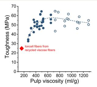
**Fig. 11** The modulus of toughness of the loncell fibers as a function of pulp viscosity (closed circles: HWPHK pulps; open circles: SWS-IP pulps).
