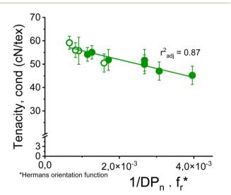
Fig. 13 Conditioned tenacity of loncell fibers with titers of  $1.21\pm0.10$  dtex made from SWS-IP (open circles) and HWPHK pulps (closed circles) as a function of the reciprocal DP<sub>n</sub> times the Hermans orientation function  $f_r$ .
