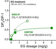
Fig. 1 The chain scission rate of cellulose during the acid (left) and endoglucanase treatment (right).
