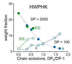
Fig. 3 The cellulose chain scission rate as a function of molecular weight fractions: left: SWS-IP pulp, right: HW-PHK pulp. Green symbols: endoglucanase (EG), blue symbols: acid (A) treatments. Full symbols, circles and diamonds: DP > 2000 fractions; open symbols, circles and diamonds: DP < 100 fractions.
