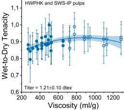
Fig. 10 Strength properties of the spun fiber as a function of pulp viscosity. Left: conditioned tenacity, right: ratio between conditioned and wet tenacities (closed circles: HWPHK pulps; open circles: SWS-IP pulps).
