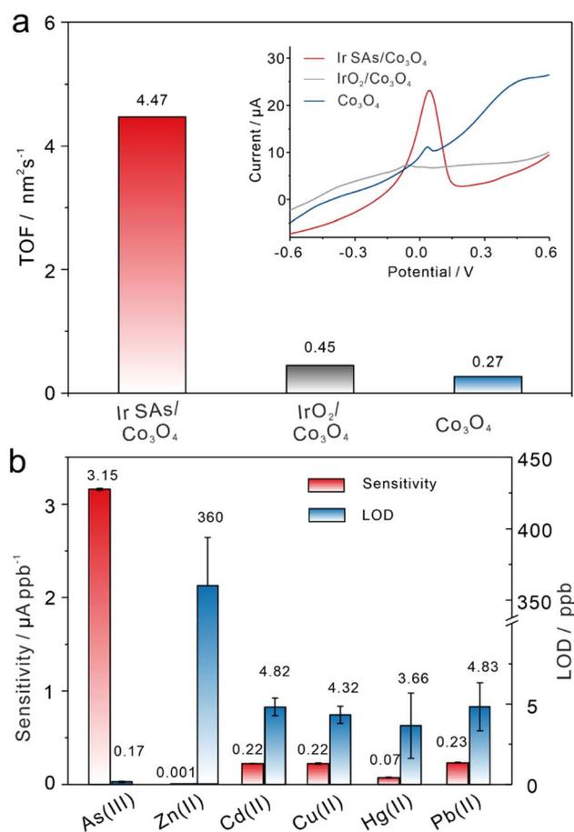
Fig. 2 Electrochemical detection of As(III) and selectivity tests toward common heavy metal ions. (a) Comparison of TOF and LSV responses toward 10 ppb As(III) (inset) on Ir SAs/Co<sub>3</sub>O<sub>4</sub>, IrO<sub>2</sub>/Co<sub>3</sub>O<sub>4</sub>, and Co<sub>3</sub>O<sub>4</sub> modified electrodes under the same conditions. (b) Sensitivity and LOD of Ir SAs/Co<sub>3</sub>O<sub>4</sub> toward different HMIs.
