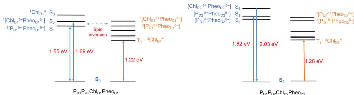
Fig. 6 Schematic representation of selected low-energy singlet and triplet excitations for the  $\text{P}_{\text{D1}}\text{P}_{\text{D2}}\text{Chl}_{\text{D1}}\text{PheO}_{\text{D1}}$  and  $\text{P}_{\text{D1}}\text{P}_{\text{D2}}\text{Chl}_{\text{D2}}\text{PheO}_{\text{D2}}$  tetrameric assemblies computed using (TDA)-TDDFT with QM/MM at the  $\omega\text{B97X-D3BJ/def2-TZVP}$  level of theory.
