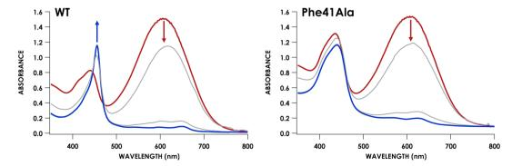
Fig. 7 Full-wavelength UV/vis absorption traces showing the reactions of 12  $\mu$ M WT (left) or Phe41Ala (right) cyt P460 with 70  $\mu$ M DCPIP and 10 mM NH<sub>2</sub>OH. The red trace is before NH<sub>2</sub>OH addition and the blue trace is the end of the reaction. Grey traces represent scans after NH<sub>2</sub>OH addition collected every 6 seconds.
