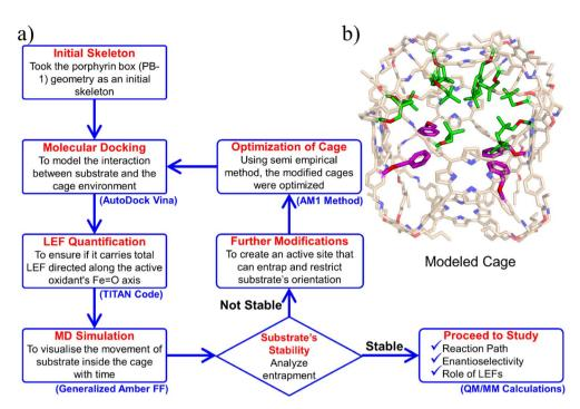
Fig. 2 (a) A flowchart of the protocol to engineer the porphyrin box for the substrate and active oxidant HM1. (b) Modeled cage, here modifications are highlighted in green.
