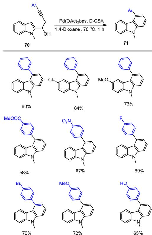
Scheme 48 Synthesis of carbazoles using Pd(OAc)<sub>2</sub>bpy catalyst.
