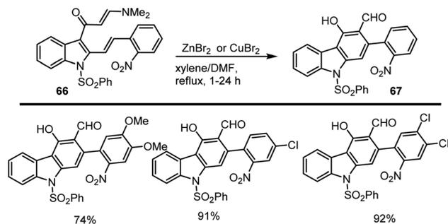
Scheme 46 Lewis acid mediated synthesis of tri-substituted carbazole.
