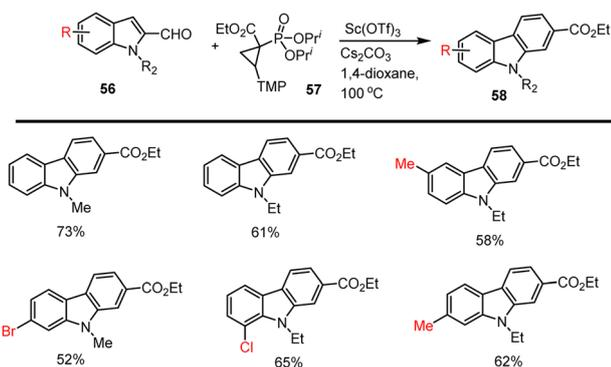
Scheme 39 Synthesis of carbazoles used by  $\text{Sc}(\text{OTf})_3$ .
