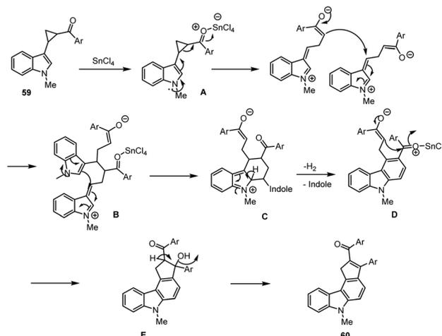
Scheme 41 Proposed mechanism of domino carbocationic rearrangement.
