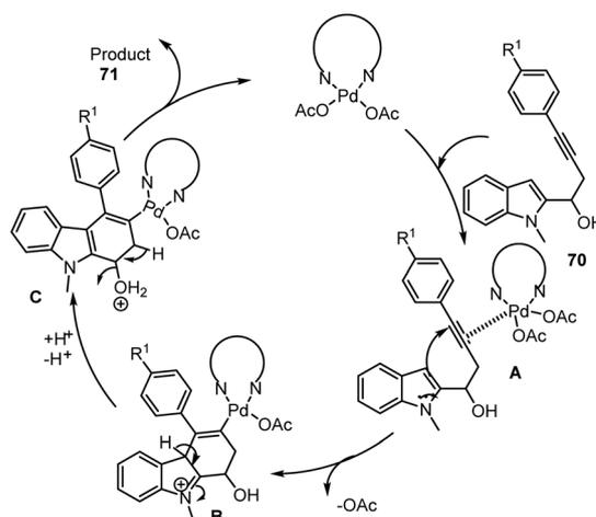
Scheme 49 Plausible mechanism for Pd(OAc)<sub>2</sub>bpy-catalyzed synthesis of carbazoles.
