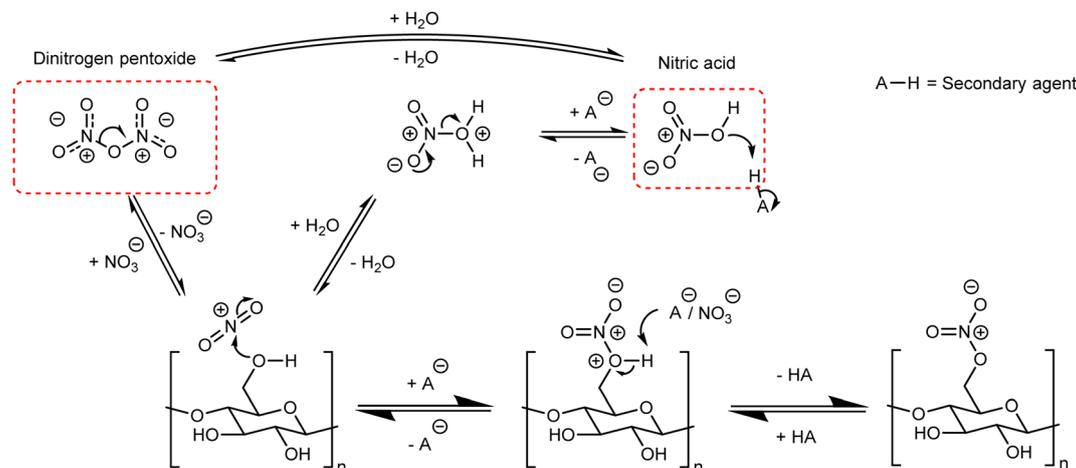
Fig. 5 General mechanism for the nitration of cellulose.
