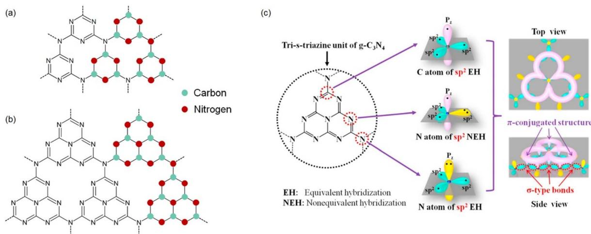
Fig. 1 Schematic illustration of chemical structure of  $g\text{-C}_3\text{N}_4$ : (a) triazine structure and (b) tri- $s$ -triazine structure. (c) Hybrid structure and  $\pi$ -conjugated structure of the tri- $s$ -triazine unit of  $g\text{-C}_3\text{N}_4$ . Reproduced from ref. 23 with permission. Copyright 2019, Elsevier.
