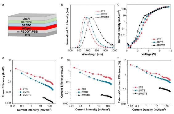
Fig. 4 (a) Schematic of the device structure of the non-doped OLEDs. (b) Normalized electroluminescence (EL) spectra of the devices based on 2TB, 2MTB, and 2MOTB. (c) Current density -voltage characteristics. (d) power efficiency, (e) current efficiency, and (f) EQE versus current density curves of the devices
