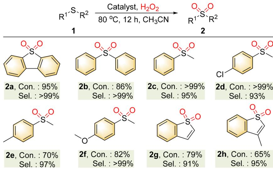
**Scheme 2** Substrate expansion for catalytic oxidation of thioether by **1**.
