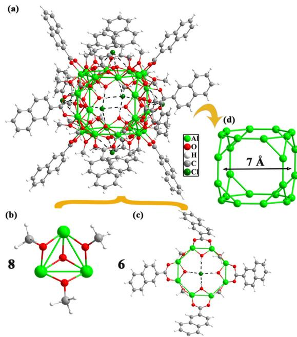
**Fig. 2** (a) Molecular structures of  $\text{Al}_{24}$ . (b) and (c) The  $[\text{Al}_3(\text{OH})(\text{CH}_3\text{O})_3]$  and  $[\text{Al}_8(\text{OH})_4(\text{CH}_3\text{O})_4(\text{NAP})_4]$  building blocks. (d) The 24-nuclearity Al metallic skeleton with a truncated hexahedral geometry (green: Al; red: O; grey: C; dark green: Cl; white: H).
