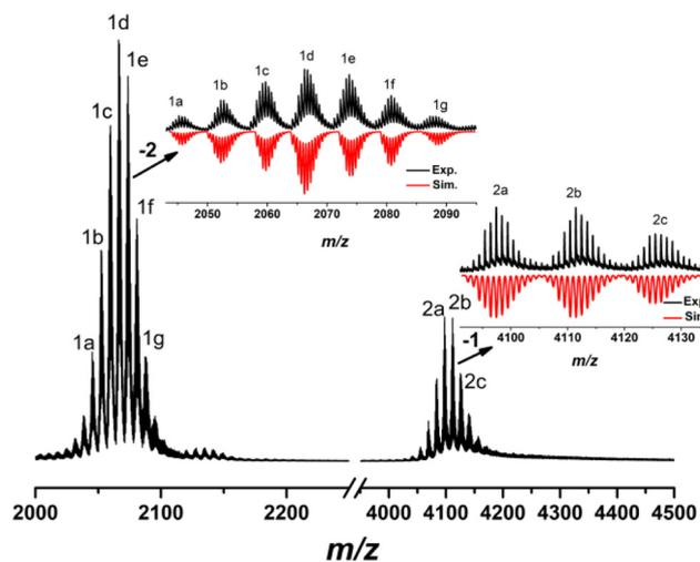
**Fig. 4** The negative-ion ESI-MS of Al<sub>24</sub> in CH<sub>3</sub>OH/CH<sub>2</sub>Cl<sub>2</sub>. Inset: the experimental isotopic pattern (block) and simulated (red) data.
