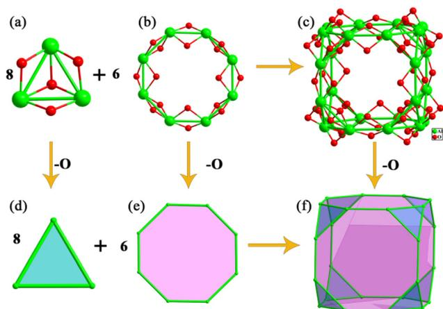
**Fig. 3** (a) and (b) [Al<sub>3</sub>(OH)O<sub>3</sub>] and [Al<sub>6</sub>(OH)<sub>8</sub>O<sub>4</sub>] building units. (c) The Al/O core of Al<sub>24</sub>. (d) and (e) The simplified Al<sub>3</sub> triangle (blue) and Al<sub>6</sub> octagon (purple). (f) The Archimedean polyhedron of Al<sub>24</sub> metallic core (green: Al; red: O).
