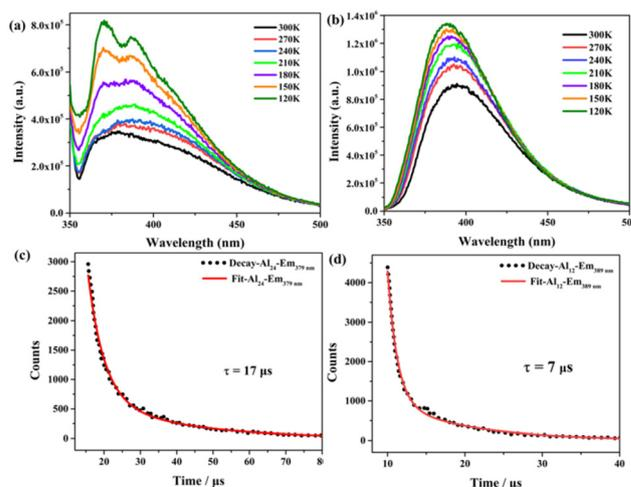
Fig. 8 The temperature-dependent luminescence spectra of Al<sub>24</sub> (a) and Al<sub>12</sub> (b) from 300 K to 120 K. Luminescence lifetimes of Al<sub>24</sub> (c,  $\lambda_{em}$  = 379 nm) and Al<sub>12</sub> (d,  $\lambda_{em}$  = 389 nm) at room temperature.
