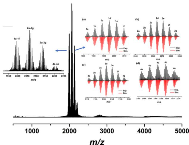
Fig. 5 The positive-ion ESI-MS of  $\text{Al}_{24}$  in  $\text{CH}_3\text{OH}/\text{CH}_2\text{Cl}_2$ . Left inset: the experimental isotopic pattern. Right inset: the experimental isotopic pattern (block) and simulated (red) data.
