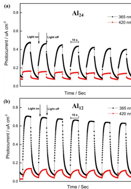
Fig. 7 Transient photocurrent responses of Al<sub>24</sub> (a) and Al<sub>12</sub> (b).
