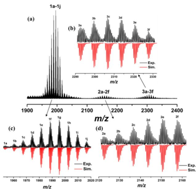
Fig. 6 (a) The positive-ion ESI-MS of  $\text{Al}_{12}$  in  $\text{CH}_3\text{OH}/\text{CH}_2\text{Cl}_2$ . The experimental isotopic pattern (block) and simulated (red) data for 1 group (c), 2 group (d), and 3 group (b).
