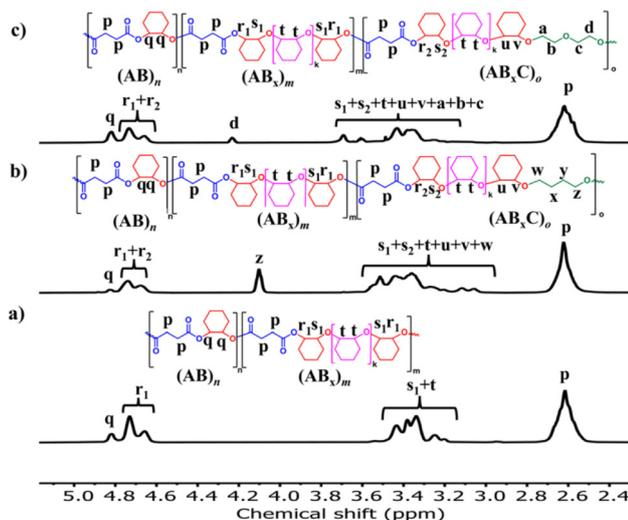
**Fig. 6**  $^1\text{H}$  NMR spectra (600 MHz,  $\text{CDCl}_3$ , 30 °C) of (a)  $\text{AB}_x$  copolymer (Table 1, entry 6, for comparison); (b)  $\text{AB}_x\text{C}$  copolymer; C = THF (Table 2, entry 4); and (c)  $\text{AB}_x\text{C}$  copolymer; C = OX (Table 2, entry 9).
