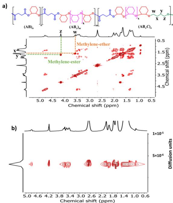
**Fig. 7** COSY and DOSY-NMR spectra (600 MHz,  $\text{CDCl}_3$ , 30 °C) of the copolymer from ROCOP of SA, CHO and THF using a SA/CHO/THF/SnOct<sub>2</sub> molar ratio of 50 : 150 : 150 : 1 (Table 2, entry 3).
