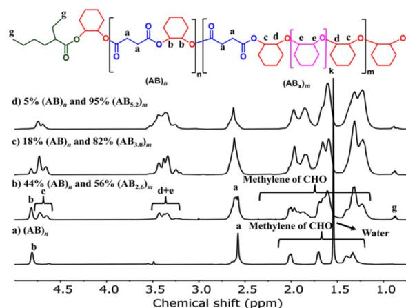
Fig. 2  $^1\text{H}$  NMR spectra (600 MHz,  $\text{CDCl}_3$ , 30 °C) of the copolymer from ROCOP of SA and CHO having different AB and  $AB_x$  components.
