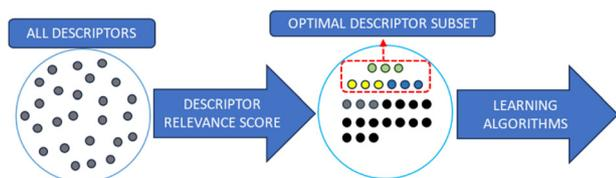
**Fig. 3** Descriptor selection workflow. The relevance score for each descriptor is computed. Based on the score, descriptors are ranked, and an optimal descriptor subset is identified. This subset is then fed into machine learning algorithms.
