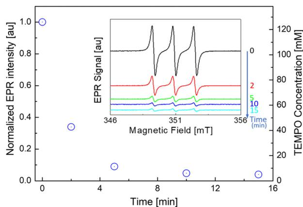
**Fig. 4** EPR monitoring of the TEMPO concentration for the reaction of C18 with 4 mol% TEMPO and 2 mol% DCP at 150 °C: TEMPO-normalized EPR intensities ( $I/I_0 = I(t)/I(t=0)$ ) were obtained at  $t = 0, 2, 5, 10$  and 15 min with corresponding EPR signals (inset).
