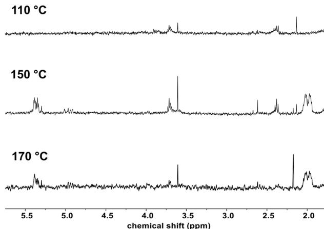
Fig. 2 <sup>1</sup>H NMR spectra (CDCl<sub>3</sub>) of the reaction mixture of C18 with 4 mol% of TEMPO in the presence of 2 mol% of DCP at different temperatures.
