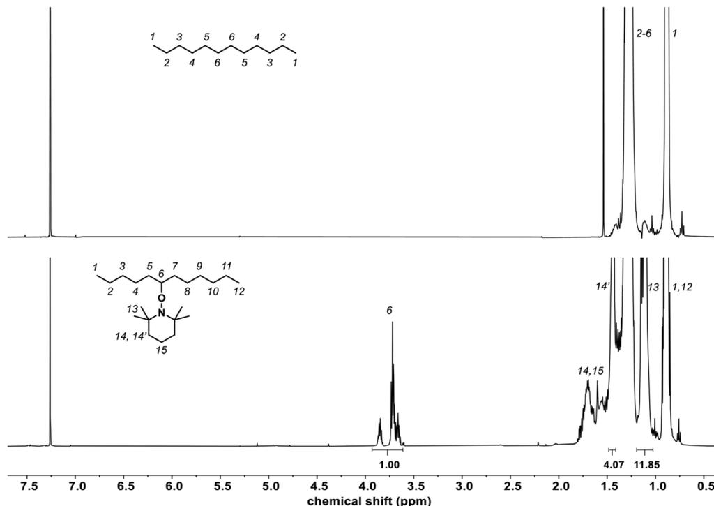
**Fig. 3**  $^1\text{H}$  NMR spectra ( $\text{CDCl}_3$ ) of C12 (top) and TEMPO-grafted C12 (bottom) formed by the reaction of C12 with TEMPO (4 mol%) and DCP (2 mol%) at 150 °C after 19 h and concentrated by distillation. The NMR assignment of TEMPO-grafted C12 is illustrated with the TEMPO grafted in the center, but it could be on any carbon of the C12 chain.
