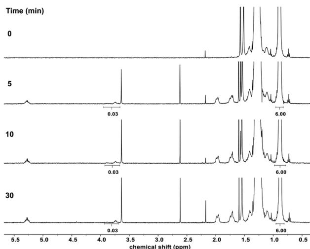
**Fig. 5** Monitoring of the grafting of diTEMPO (4 mol%) on C18 in the presence of DCP (4 mol%) at 150 °C. The peak at 0.9 ppm was taken as a reference for all the terminal methyl groups of modified and unmodified C18, while the peak at 3.7 ppm corresponded to the proton on the carbon onto which a TEMPO group was grafted.
