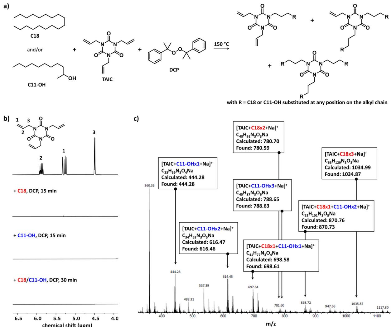
**Fig. 1** Coupling of TAIC (1 mol%) on C18 and/or C11-OH in the presence of DCP (0.5 mol%) at 150 °C: (a) reaction scheme, (b) monitoring of the consumption of the allyl group using <sup>1</sup>H NMR spectroscopy in CDCl<sub>3</sub> (full spectra in ESI, Fig. S1†), and (c) ESI-MS spectrum of the raw product obtained from the reaction performed on the mixture of C18 and C11-OH (1/1) (zoom on the molecular peaks and their simulation in ESI, Fig. S2†).
