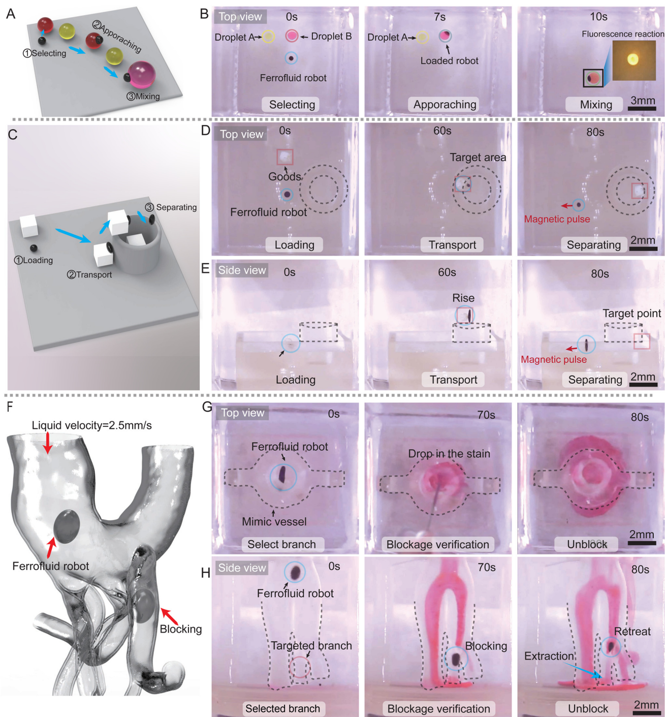
Fig. 7 Experimental validation of multifunctionality in ferrofluidic robots. (A) Conceptual illustration of a ferrofluidic robot employed for controlled chemical micro-reactions via droplet mixing. (B) The process and fluorescence imaging results of a fusion reaction, orchestrated by a ferrofluidic robot, between droplets containing disparate solvents. (C) Schematic representation of a ferrofluidic robot purposed for micro-operation. (D) Top view and (E) primary view of a ferrofluidic robot controlling and conveying goods to a designated area, demarcated by the black dashed contour line. (F) Conceptual depiction of a ferrofluidic robot for selective blood vessel occlusion. (G) Top view and (H) primary view of the experimental procedure illustrating controllable blood vessel blockage facilitated by a ferrofluidic robot.
