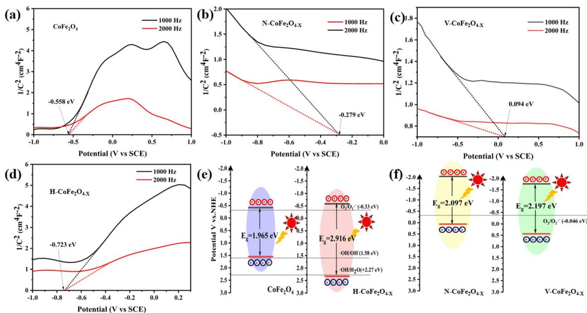
**Fig. 6** Mott Schottky curves for (a)  $\text{CoFe}_2\text{O}_4$ , (b)  $\text{N-CoFe}_2\text{O}_{4-x}$ , (c)  $\text{V-CoFe}_2\text{O}_{4-x}$ , and (d)  $\text{H-CoFe}_2\text{O}_{4-x}$ ; (e) energy band diagrams of n-type semiconductor photocatalytic samples  $\text{CoFe}_2\text{O}_4$  and  $\text{H-CoFe}_2\text{O}_{4-x}$  and (f) energy band diagrams of p-type semiconductor photocatalytic samples  $\text{N-CoFe}_2\text{O}_{4-x}$  and  $\text{V-CoFe}_2\text{O}_{4-x}$ .
