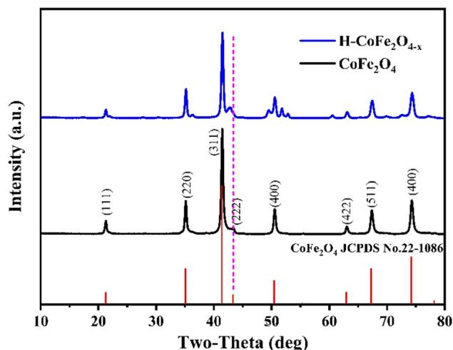
**Fig. 4** XRD patterns of CoFe<sub>2</sub>O<sub>4</sub> and H-CoFe<sub>2</sub>O<sub>4-x</sub>.
