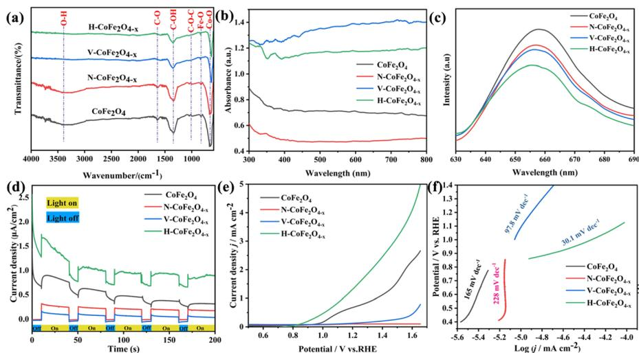
**Fig. 5** (a) FT-IR, (b) diffuse reflectance UV-vis spectrum, (c) PL spectra ( $\lambda = 420$  nm), (d) photocurrents under visible light irradiation, (e) linear sweep voltammetry (LSV) and (f) Tafel images of  $\text{CoFe}_2\text{O}_4$ ,  $\text{N-CoFe}_2\text{O}_{4-x}$ ,  $\text{V-CoFe}_2\text{O}_{4-x}$ , and  $\text{H-CoFe}_2\text{O}_{4-x}$ .
