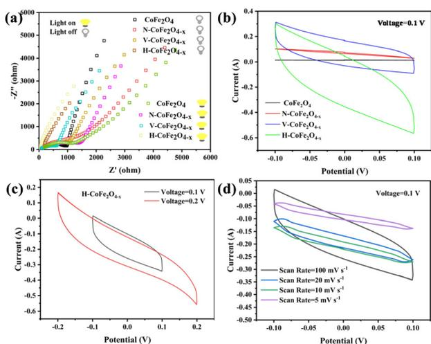
**Fig. 7** (a) Electrochemical impedance spectroscopy (EIS), (b) cyclic voltammetry (CV) curves of four samples, (c) CV curves of  $\text{H-CoFe}_2\text{O}_{4-x}$  at different voltages ( $-0.1$ – $0.1$ , and  $-0.2$ – $0.2$  V) and (d) CV curves of  $\text{H-CoFe}_2\text{O}_{4-x}$  at different scan rates (5, 10, 20, and 100  $\text{mV s}^{-1}$ ).
