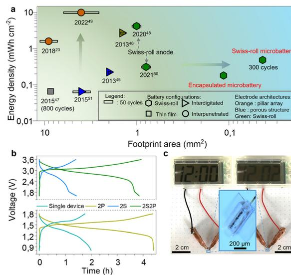
**Fig. 4** Comparison of Swiss-roll microbattery performance. (a) Comparison of areal energy density, footprint area, and cycling performance of Swiss-roll microbatteries with previously reported ones. (b) GCD curves of microbatteries connected in series and parallel. (c) Digital photographs of Swiss-roll microbattery powering a digital watch for two min (inset is the encapsulated Swiss-roll microbattery).
