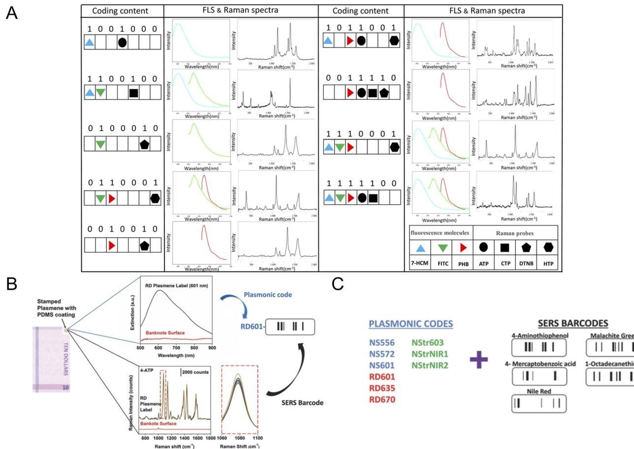
**Fig. 8** (A) Raman–fluorescence combined encoding for security labels; Raman–absorption combined encoding for security labels. Reproduced with permission from ref. 60. Copyright 2016 American Chemical Society. (B) Schematic diagram of the encoding source; (C) double layer encoding – plasmonic encoding and Raman encoding. Reproduced with permission from ref. 61. Copyright 2015 John Wiley & Sons, Inc.
