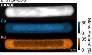
Fig. 1 Shape and composition of Cu and Cu-CuPd NRs. TEM image of representative (A) Cu NRs and Cu-CuPd NRs with varying concentrations of Pd precursor resulting in NRs with Pd mass percent of (B) 22, (C) 42, and (D) 46%. (E) HAADF signal and STEM-EDS elemental maps for Cu and Pd in a Cu-CuPd NR from the batch containing 46% Pd by mass
