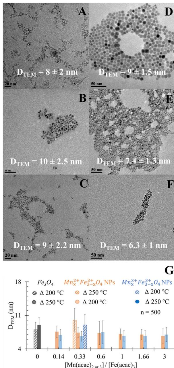
Fig. 1 TEM images for the spherical (A) undoped  $Fe_3O_4$  NPs, (B)  $Mn_xFe_{3-x}O_4$  of precursor ratio  $[Mn(acac)_2]/[Fe(acac)_3] = 0.33$ , (C)  $[Mn(acac)_3]/[Fe(acac)_3] = 0.33$  prepared at 200 °C as reaction temperatures, (D) undoped  $Fe_3O_4$  NPs and (E) and (F)  $Mn_xFe_{3-x}O_4$  NPs prepared with the same precursor ratio but at 250 °C. (G) Impact of reaction temperatures on  $D_{TEM}$  of  $Mn_xFe_{3-x}O_4$  NPs prepared from  $[Mn(acac)_2]/[Fe(acac)_3] = 0.33$ . \* $P < 0.05$ .
