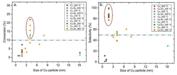
Fig. 13 (a) Conversion of CO<sub>2</sub> versus size of Cu particle. (b) Selectivity towards methanol versus size of Cu particle. Blue dashed lines represent 10% conversion and 50% selectivity
