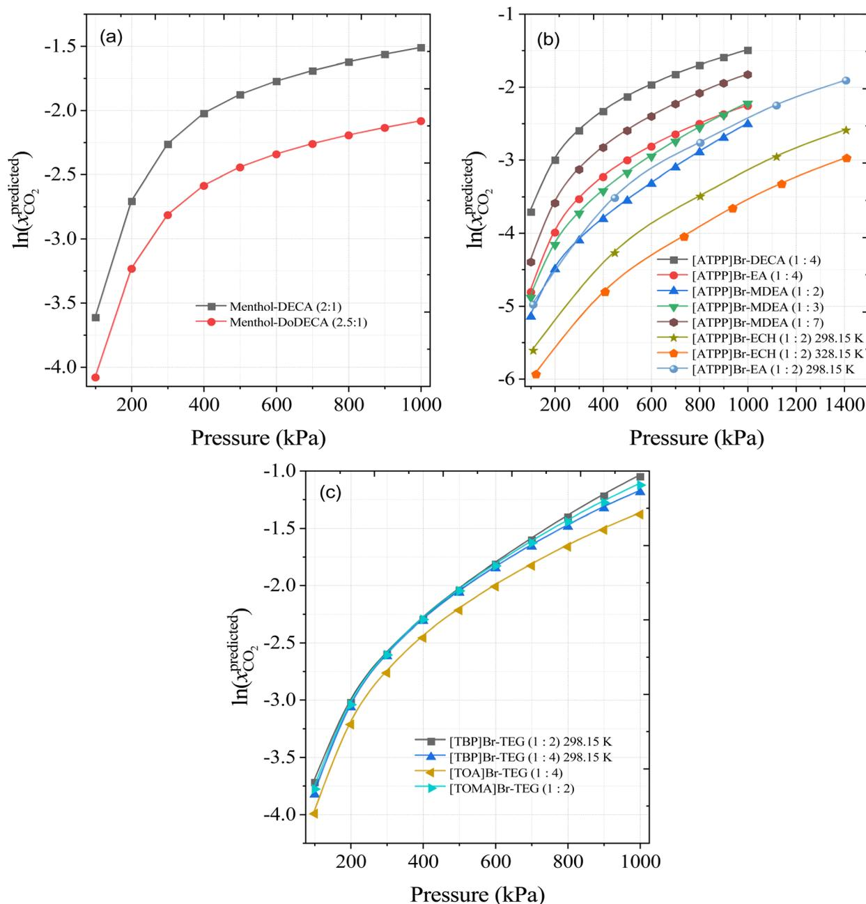
**Fig. 12** Development of new DESs combination for improving CO<sub>2</sub> solubilities using the machine learning model, DES composed of (a) menthol as HBA and decanoic acid and dodecanoic acid as HBDs, (b) [ATPP]Br HBA and EA, DECA, MDEA, and ECH are HBDs, and (c) [TBP]Br, [TOA]Br, and [TOMA]Br are HBAs with TEG HBD.
