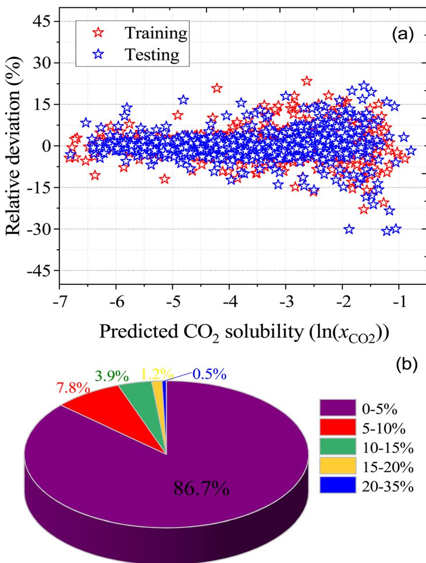
Fig. 7 (a) relative deviation between the experimental and predicted CO<sub>2</sub> solubilities in DES, and (b) the distribution of the absolute relative deviation in different deviation ranges.
