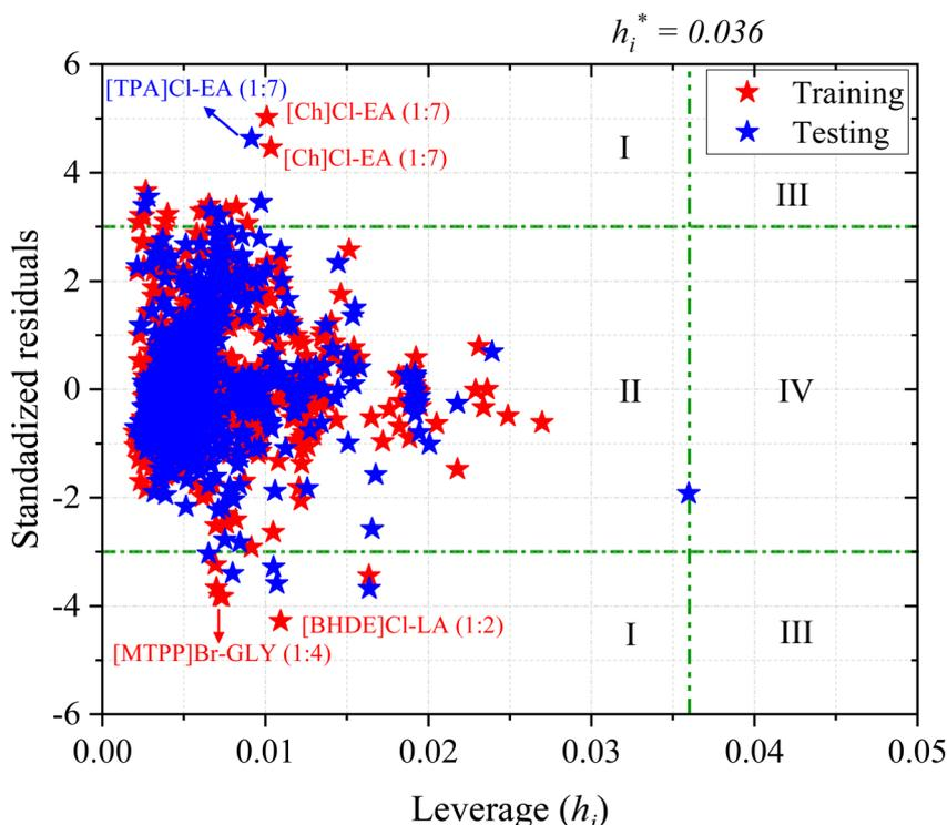
Fig. 8 Williams plot (standardized residual vs. leverage) of the total set of ML model for the CO<sub>2</sub> solubility in DESs.
