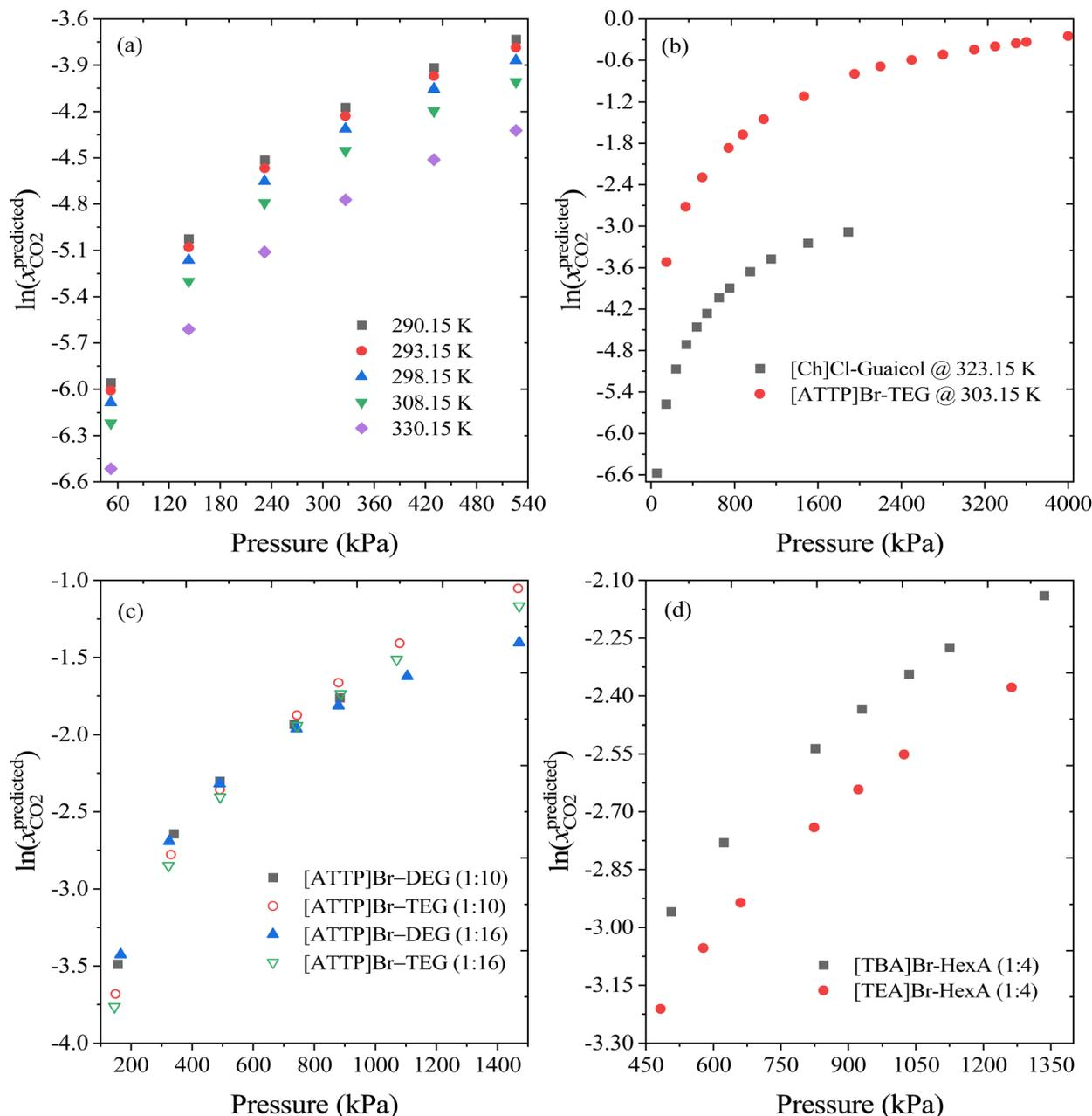
**Fig. 10** ANN-based machine learning predicted CO<sub>2</sub> solubilities in (a) [Ch]Cl-Guaiacol (1:4) at different temperatures, (b) [Ch]Cl and [ATTP]Br-based DES at different pressures, and (c and d) effect of molar ratio, HBDs and HBAs on CO<sub>2</sub> solubility.
