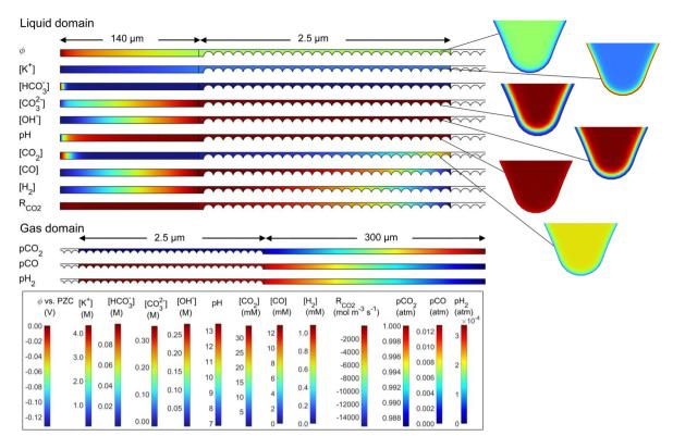
Potential, concentrations, and partial pressures for the 50%-filled case with a cathode potential of -1.1 V vs. RHE and a 0.1 M KHCO<sub>3</sub> electrolyte.
