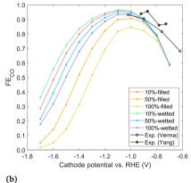
Fig. 7 (a) Geometric CO current density for modeled cases and experimental data from Verma et al., 38 Yang et al., 4 and García de Arquer et al. 24 and (b) overall Faradaic efficiency to CO
