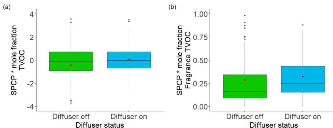
Fig. 8 (a) Calculated total SPCP values differentiated by diffuser status, and (b) SPCP from fragrance species, where data was available. The SPCP \* mole fraction product is given as a dimensionless quantity, as SPCP is expressed in units of  $\text{ppb ppb}^{-1}$ . Outliers below  $-4$  and above  $+4$  for (a) and outliers above  $1$  for (b) were removed from the graphic to aid presentation, but were included in the calculation of quartiles and median values.
