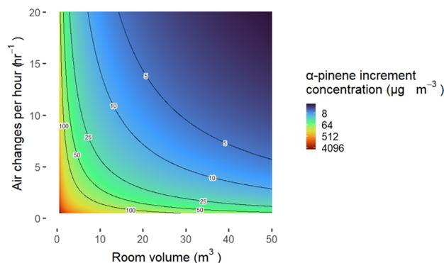
Fig. 7 A raster plot overlaid with contour lines showing the  $\alpha$ -pinene increment expected for different room volumes and ventilation rates. A continuous colour scale was applied to  $\alpha$ -pinene increment values, and the scale was transformed on a  $\log_2$  scale to aid visualisation.
