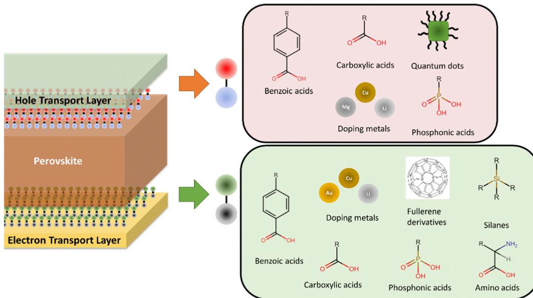
Fig. 5 Summary of materials employed for interface optimisation in perovskite solar cells at the electron transport layer/perovskite interface and the hole transport layer/perovskite interface.
