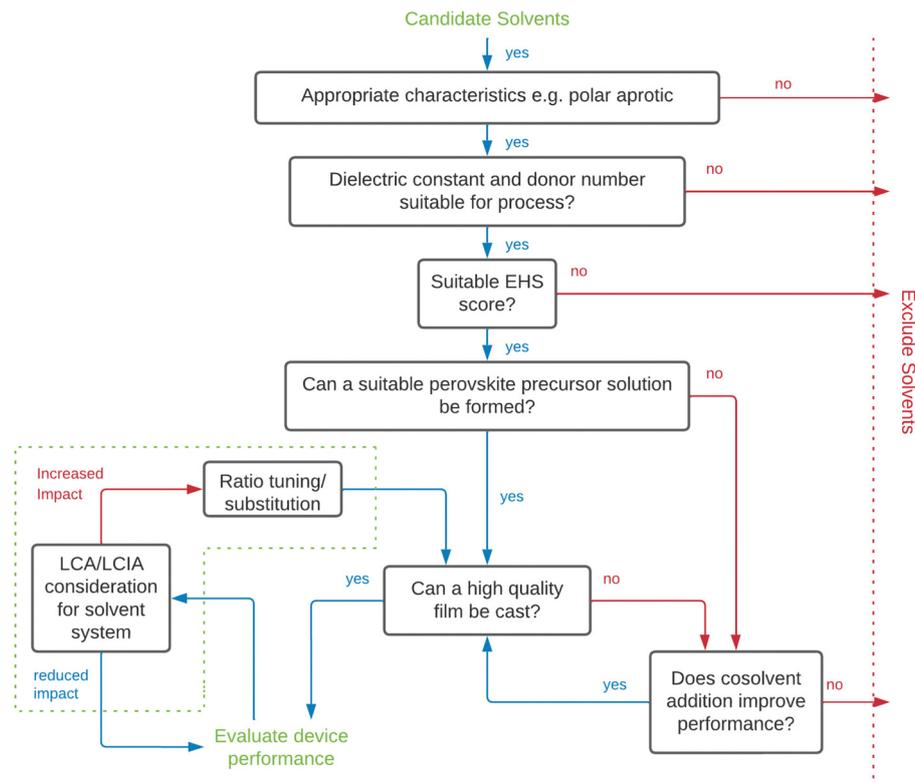
Fig. 6 Solvent selection decision tree for screening and evaluation of alternative solvents for perovskite deposition (adapted from Doolin *et al.*).<sup>275</sup> EHS – Environmental, health and safety, LCA – life cycle assessment, LCIA – life cycle impact assessment, MAPbI<sub>3</sub> – methylammonium lead triiodide.
