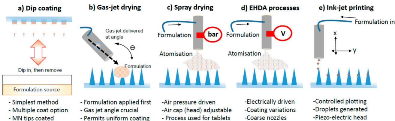
**Fig. 3** Illustrated examples of techniques used to coat MNs. (a) Dip coating; (b) gas-jet drying; (c) spray drying; (d) EHDA processes; (e) ink-jet printing. Reprinted with permission from MDPI,<sup>20</sup> Copyright 2015.
