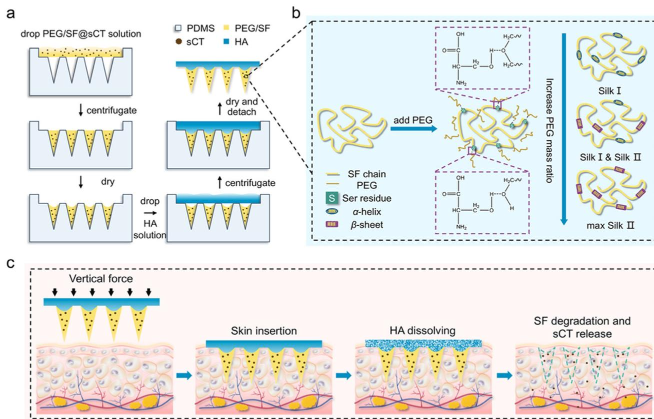
**Fig. 5** Schematic illustrations of the fabrication process of HA-PEG/SF@sCT MNs (a), PEG-induced conformational transition of SF (b), and transmucosal delivery of sCT using the HA-PEG/SF@sCT MNs (c). Silk fibroin (SF); poly(ethylene glycol) (PEG); salmon calcitonin (sCT). Reprinted with permission from American Chemical Society,<sup>38</sup> Copyright 2023.
