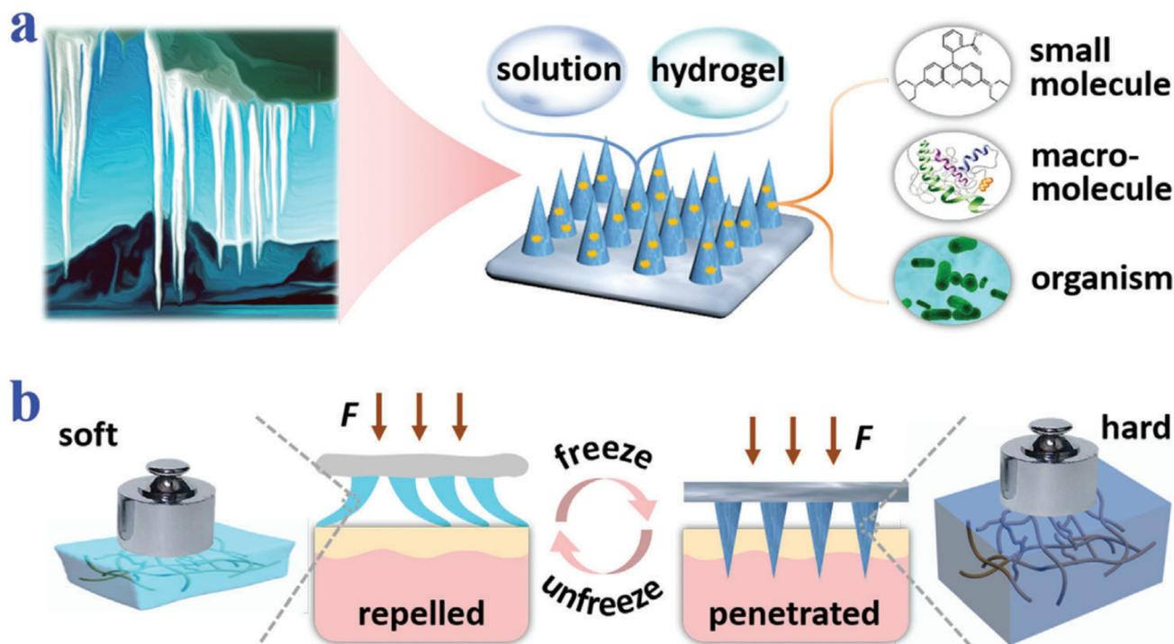
**Fig. 8** Schematic illustrations of compositions and properties of ice MNs. (a) Ice-formation-inspired ice MNs can be made from soft materials such as solutions and hydrogels, and can carry diverse actives including small molecules, macromolecules, and living organisms. (b) Scheme of transformation from softness to hardness realized by freezing processes. Reprinted with permission from American Chemical Society Advanced Science published by Wiley-VCH GmbH,<sup>61</sup> Copyright 2021.
