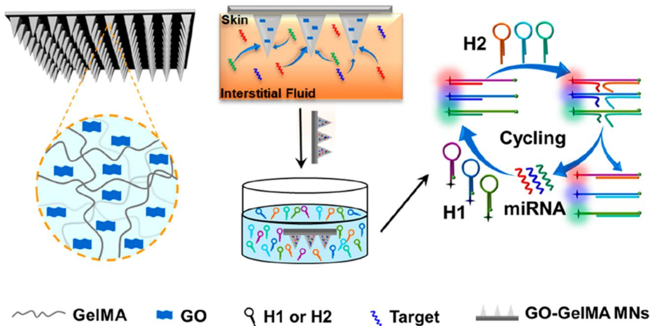
Fig. 7 Schematic illustration of GO-GelMA MNs used for interstitial fluid extraction and the detection of miRNA. Reprinted with permission from American Chemical Society,<sup>53</sup> Copyright 2023.
