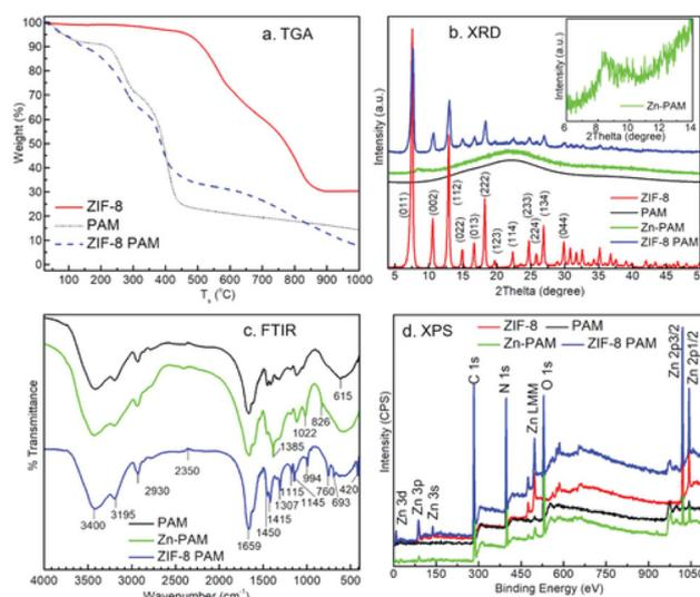
**Fig. 7** Different characterisation methods used to provide support to the successful synthesis of ZIF-8/PAM hybrid. (a) TGA, (b) powder XRD, (c) FT-IR, (d) XPS. Reproduced from ref. 63 with permission from John Wiley and Sons, copyright 2019.
