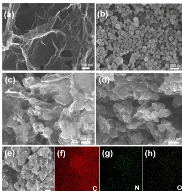
**Fig. 6** SEM images of (a) Graphene hydrogel (b) cZIF-8 (c) MOF-hydrogel (d) Quantum dots on MOF-hydrogel. (e-h) Elemental mapping of the Quantum dots on MOF-hydrogel. Reproduced with permission from ref. 72. Copyright 2020 Elsevier.
