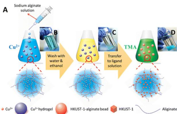
**Fig. 5** (A) Schematic of the preparation of the MOF–alginate composite. Photographs of (B) alginate hydrogels cross-linked to  $\text{Cu}^{2+}$ , (C) alginate metal hydrogels after washing, (D) MOF–hydrogel hybrids. Reprinted with permission from ref. 62. Copyright 2016 American Chemical Society.
