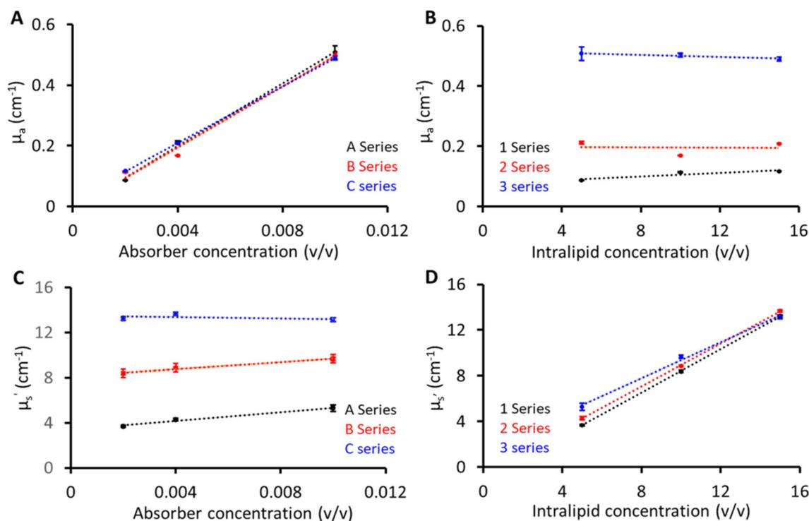
**Fig. 3** Results of linearity tests at 830 nm. (A) Absorption coefficient  $\mu_a$  as a function of the added absorber (B) impact of different amounts of added scatterers on  $\mu_a$ . (C) Reduced scattering coefficient  $\mu'_s$  as a function of the added absorber. (D) Impact of different amounts of added scatterers on  $\mu'_s$ .
