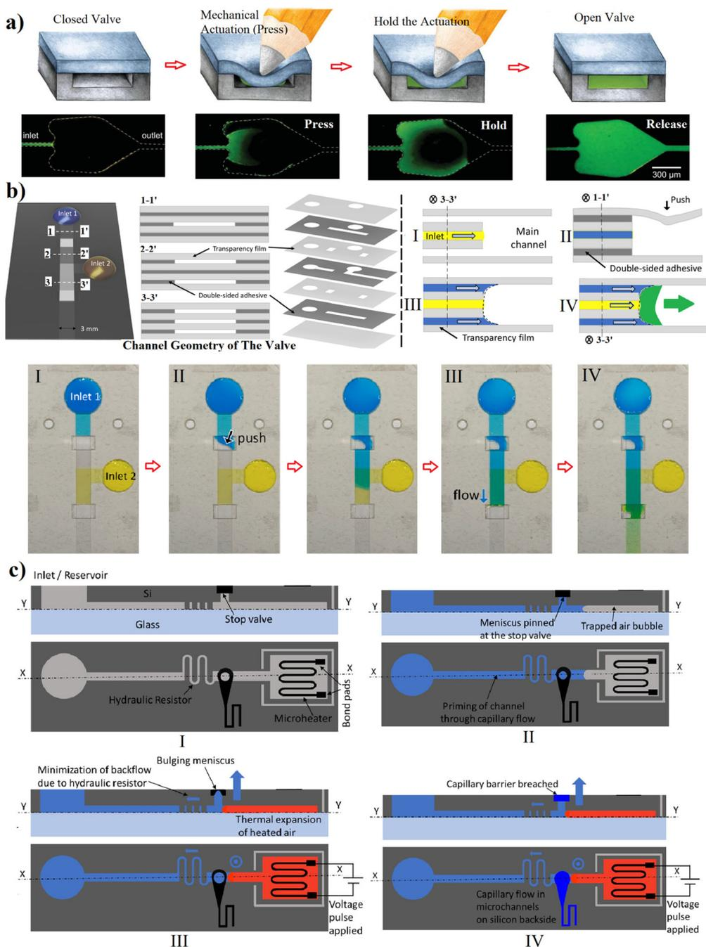
**Fig. 6** Assisted actuation of capillary valves based on: (a and b) manual (mechanical push) actuation,<sup>24,30</sup> and (c) thermo-pneumatic-pressure,<sup>31</sup> it was filled with the capillary flow and waiting to be triggered, a voltage was provided to heat up and expand the trapped air bubble, and valve is actuated by breaching the capillary barrier and capillary flow commences in the microchannel. "Reprinted/adapted with permission from: (c) © 2021 Springer Nature."
