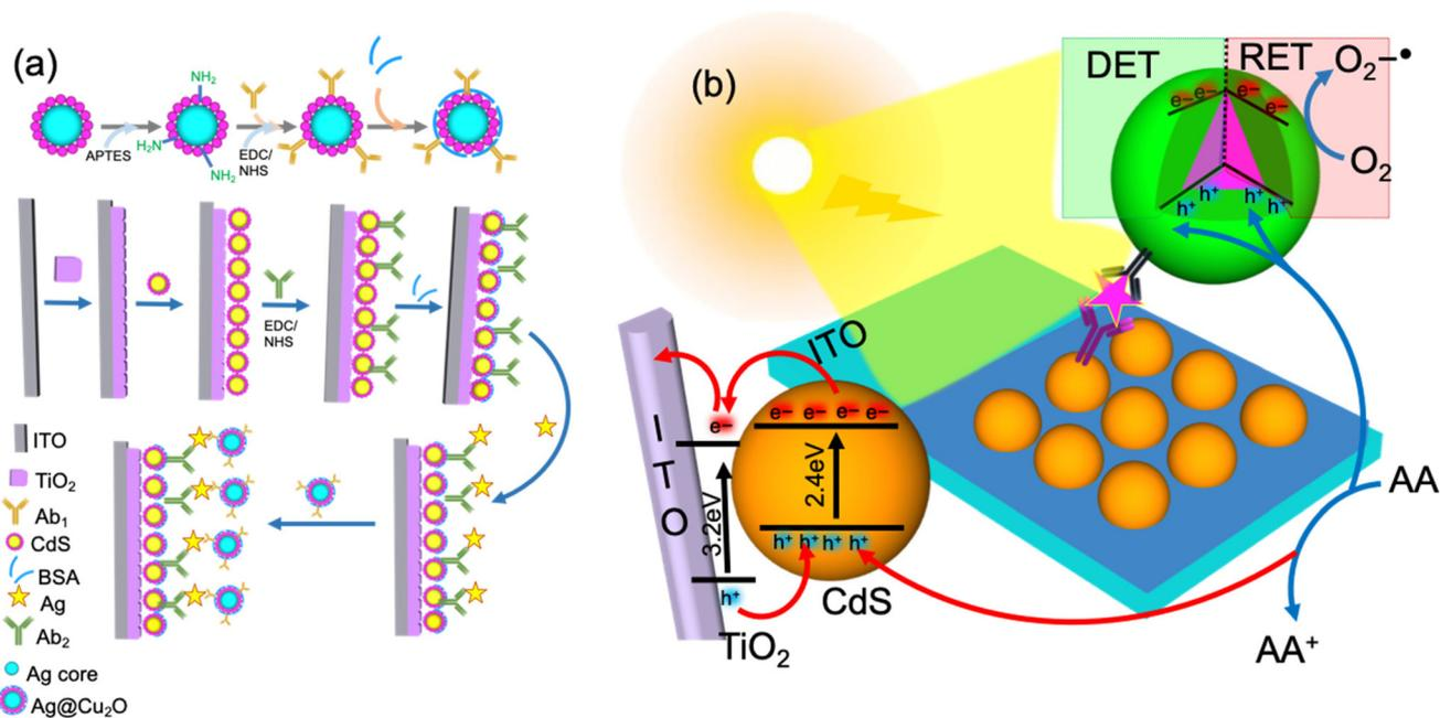
Fig. 5 The schematic illustration of: (a) the surface functionalization of an ITO/TiO<sub>2</sub>/CdS photoelectrochemical immunosensor and sandwich assay with Ag@Cu<sub>2</sub>O submicron particles for the detection of cardiac troponin, and (b) a PEC sensor showing the electron transport mechanism from CdS-sensitized TiO<sub>2</sub> nano-hybrid and Ag@Cu<sub>2</sub>O SPs.<sup>80</sup> Reprinted with permission from ref. 80 (copyright © 2018 Elsevier B.V).
