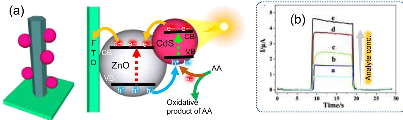
**Fig. 11** (a) Schematic illustration for the PEC sensing mechanism and (b) photocurrent for different concentrations of sulfate-reducing bacteria (SRB) (a–e = 10<sup>2</sup>–10<sup>6</sup> colony forming units per mL, respectively) at the fabricated CdS QDs/ZnO nanorod array-modified fluorine-doped tin oxide (FTO) electrode of the PEC sensor.<sup>89</sup> (a and b reprinted with permission from ref. 89 copyright © 2018 Published by Elsevier B.V.)
