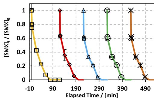
Fig. 4 Recyclability experiments of MIL88-A in the UVA/MIL88-A/PS/SMX system. Experimental conditions:  $[SMX]_0 = 5 \text{ mg L}^{-1}$ ;  $[PS]_0 = 2 \text{ mM}$ ;  $[MIL88-A] = 125 \text{ mg L}^{-1}$ ; error bars are calculated as  $ts/\sqrt{n}$ , where absent bars fall within the symbols.
