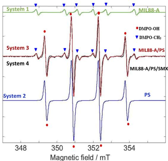
Fig. 11 EPR spectra. Green – simulated EPR spectrum for trapped methyl radicals.  $a_N = 1.58$  mT and  $a_H = 2.28$  mT. Blue – simulated EPR spectrum for trapped hydroxyl radicals.  $a_N = 1.49$  mT and  $a_H = 1.49$  mT. Red – the sum of the above two simulated trapped radical spectra. Black – experimental EPR spectrum under the following experimental conditions: [PS] = 2.5 mM, [MIL88-A] = 12.5 mg L<sup>-1</sup>, and [DMPO] = 100 mM.
