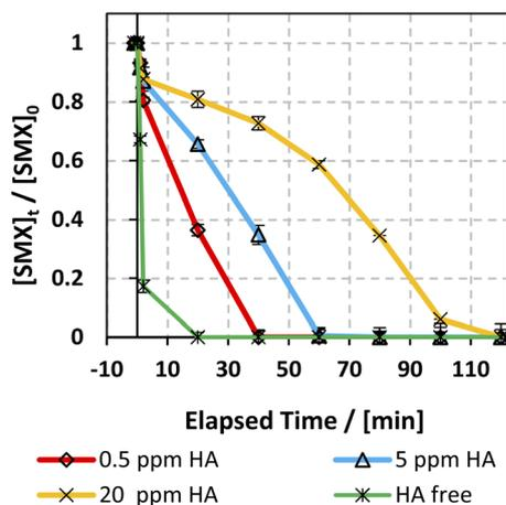
Fig. 10 Effect of HA on the degradation of SMX as a function of time (min) in the solar/MIL88-A/PS/SMX system. Experiments were done in a rotisserie shaker. Experimental conditions:  $[HA] = 0.5, 5$  and  $20 \text{ mg L}^{-1}$ ,  $[SMX]_0 = 5 \text{ mg L}^{-1}$ ,  $[PS] = 2 \text{ mM}$ , and  $[MIL88-A]_0 = 125 \text{ mg L}^{-1}$ . Error bars are calculated as  $ts/\sqrt{n}$ , where absent bars fall within the symbols.
