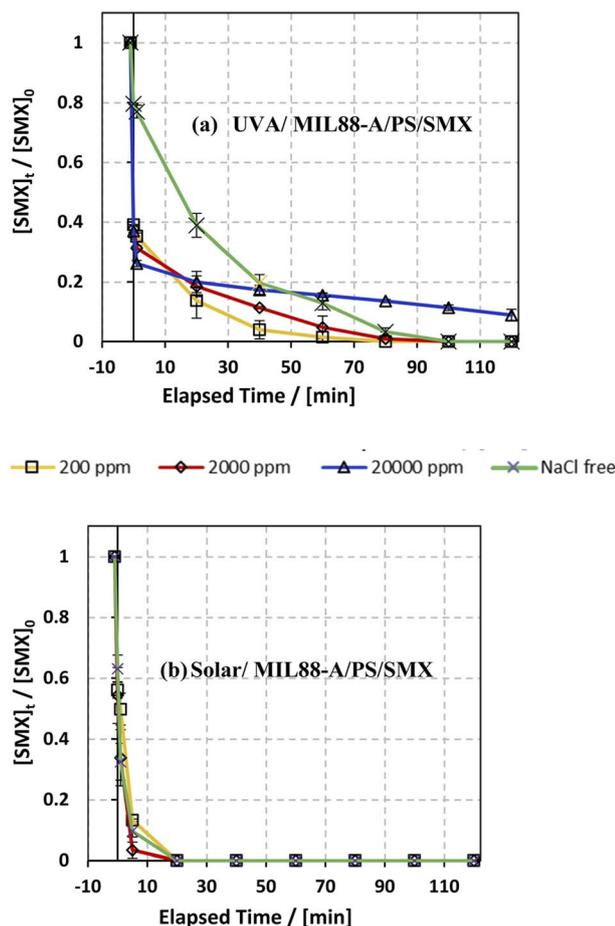
Fig. 7 Effect of  $[\text{NaCl}] = 200\text{--}20000 \text{ mg L}^{-1}$  on the degradation of SMX as a function of time (min): (a) in the UVA/MIL88-A/PS/SMX system and (b) in the solar/MIL88-A/PS/SMX system. Experimental conditions:  $[\text{SMX}]_0 = 5 \text{ mg L}^{-1}$ ,  $[\text{PS}]_0 = 2 \text{ mM}$ , and  $[\text{MIL88-A}]_0 = 125 \text{ mg L}^{-1}$ . Error bars are calculated as  $ts/\sqrt{n}$ , where absent bars fall within the symbols.
