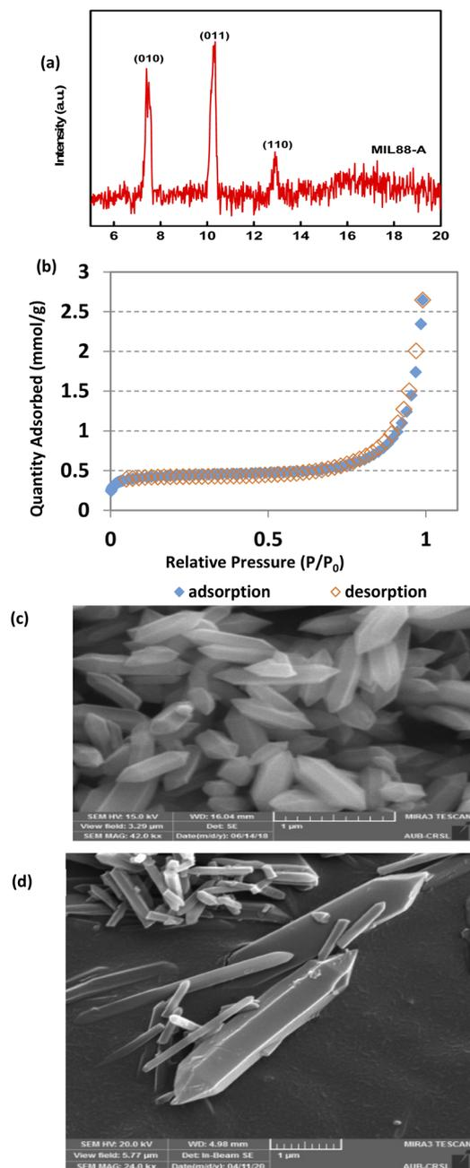
Fig. 1 SEQ Fig. \\* ARABIC Characterization of synthesized MIL88-A: (a) XRD diffraction pattern, (b) BET adsorption/desorption isotherms<sup>71</sup>, and (c and d) SEM of crystals at different magnifications.<sup>71</sup>
