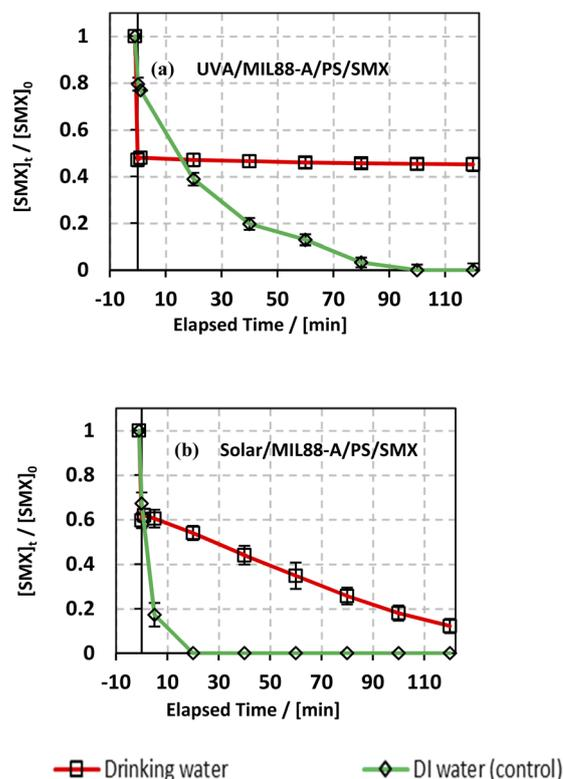
Fig. 9 Effect of drinking water and deionized water (control) on the degradation of SMX as a function of time (min): (a) in the UVA/MIL88-A/PS/SMX and (b) in the solar/MIL88-A/PS/SMX systems. Experiments were done in a rotisserie shaker. Experimental conditions: [SMX]<sub>0</sub> = 5 mg L<sup>-1</sup>, [PS] = 2 mM, and [MIL88-A]<sub>0</sub> = 125 mg L<sup>-1</sup>. Error bars are calculated as  $ts/\sqrt{n}$ , where absent bars fall within the symbols.
