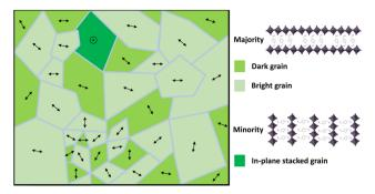
Fig. 6 Schematic of the PDMAPbl<sub>4</sub> thin film microstructure. Micro-metre sized crystallites predominantly form with layers parallel to the substrate, i.e. stacked in out-of-plane direction. These crystallites are rotationally disordered around the stacking direction (indicated by the double-arrows) and can be either bright or dark. A minor sub-population of crystallites forms with their layers perpendicular to the substrate, i.e. stacked in inplane direction
