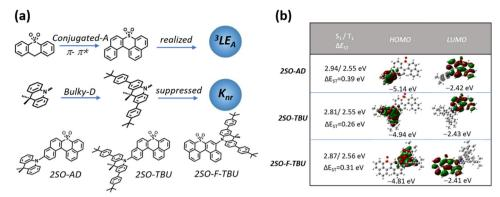
Fig. 1 (a) Schematic diagram of the molecular design strategy; (b) HOMO and LUMO electronic distributions, and the lowest singlet (S1) and triplet (T1) energy levels for 2SO-AD, 2SO-TBU and 2SO-F-TBU calculated by DFT at the B3LYP/6-31q(d,p) level.
