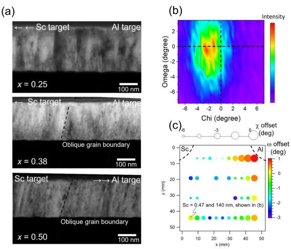
Fig. 2 Grain and crystal growth direction analysis of  $Al_{1-x}Sc_xN$ . (a) Cross-sectional TEM micrographs for Sc = 0.25 (under Al target), Sc = 0.38 (middle of library), and Sc = 0.5 (under Sc target) showing oblique grain growth. (b) XRD omega-chi plan view map for (002) wurtzite peak with respect to substrate Pt (111) normal direction. (c) Omega and chi offsets across the sample library mapping out crystal growth direction with respect to Pt (111) normal.
