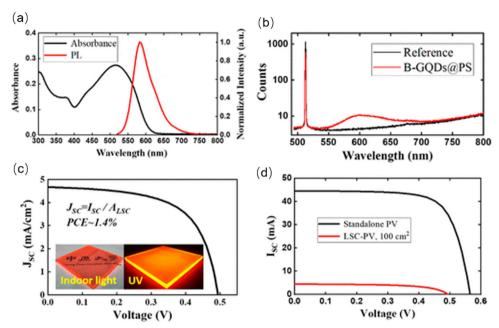
Fig. 13 (a) Absorbance and PL spectra of C-dots embedded in the PS solid matrix. (b) Experimental raw data of an absolute QY measurement. (c) The J-V curves for LSCs (100 cm<sup>2</sup>). (d) The J-V curves for standalone PVs and LSCs-PVs. Reproduced with permission from ref. 175. Copyright 2022, American Chemical Society.
