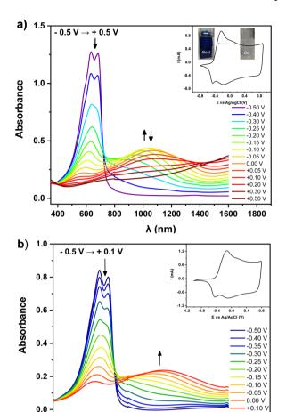
Fig. 2 CV scans and UV-vis-NIR spectra of thin films of G-PEDOT deposited on an ITO substrate, recorded for increasing electrode potential vs. Ag/AgCl pseudo-reference wire, under an inert atmosphere of argon. (a) Electrolyte: 0.1 M TBAPF<sub>6</sub>/CH<sub>3</sub>CN; (b) electrolyte: 0.1 M KCl/H<sub>2</sub>O.
