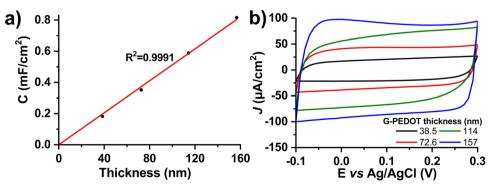
Fig. 3 Electrochemical capacitance of G-PEDOT. (a) Linear dependence of areal capacitance on the layer thickness. (b) Cyclic voltammograms  $(0.1 \text{ M KCl}, 100 \text{ mV s}^{-1})$  used for calculation of the capacitance.
