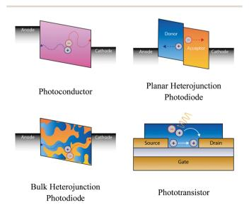
Fig. 2 The most popular device architectures of circularly polarised photodetectors. Plasmonic devices are not discussed in this perspective.
