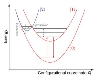
Schematic overview of the different processes determining the performance of a luminescent crossover thermometer such as Sm<sup>2+</sup> Curvy arrows indicate (multi-)phonon absorption transitions. Note that the excited state |2| has been depicted at lower configurational coordinates to match the theoretical and experimental findings for low excited 4f<sup>n-1</sup>5d<sup>1</sup> states of lanthanoid ions (see also text)
