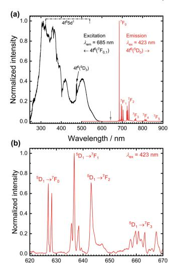
Fig. 1 (a) Photoluminescence excitation (black,  $\lambda_{em}=685$  nm) and emission (red,  $\lambda_{ex}=423$  nm) spectrum of  $SrB_4O_7$ : 0.5%  $Sm^{2+}$  at room temperature. The emission lines are assigned to the  $^5D_0 \rightarrow ^7F_J$  (J=0...6) transitions of  $Sm^{2+}$ . (b) High-resolution spectrum in the spectral range marked with the grey arrow in (a) indicates the presence of weak  $^5D_1 \rightarrow ^7F_J$  transitions.
