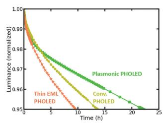
Fig. 4 Lifetime curves of the plasmonic PHOLED and reference thin and conventional EML devices aged at  $80~\text{mA}~\text{cm}^{-2}$ .
