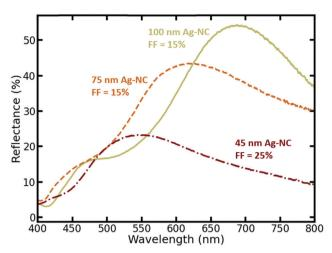
**Fig. 6** Diffuse reflectance plots of the NPA structure as measured *via* UV-vis spectroscopy for 100 nm, 75 nm, and 45 nm Ag nanocubes. As the Ag nanocube size increases the NPA resonance red-shifts and increases in intensity. The film fill fraction (FF) as measured by AFM is denoted for reference
