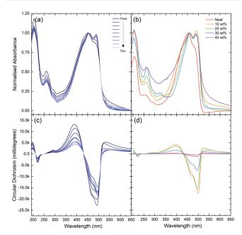
(a and b) Absorption and (c and d) circular dichroism spectra for (a and d) F8T2:10 wt% [M]-aza[6]H blends as a function of film thickness and (b and d) 100 nm thick F8T2: [M]-aza[6]H blends as a function of aza[6]H loading ratio.
