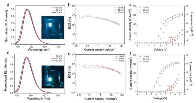
Fig. 4 EL spectra (a) (inset: emission picture of the device); EQE-current density curves (b); and current density-voltage-luminance (J-V-L) curves (c) of TTT-Ac. EL spectra (d) (inset: emission picture of the device); EQE-current density curves (e); and current density-voltage-luminance (J-V-L)curves (f) of TTT-2Ac
