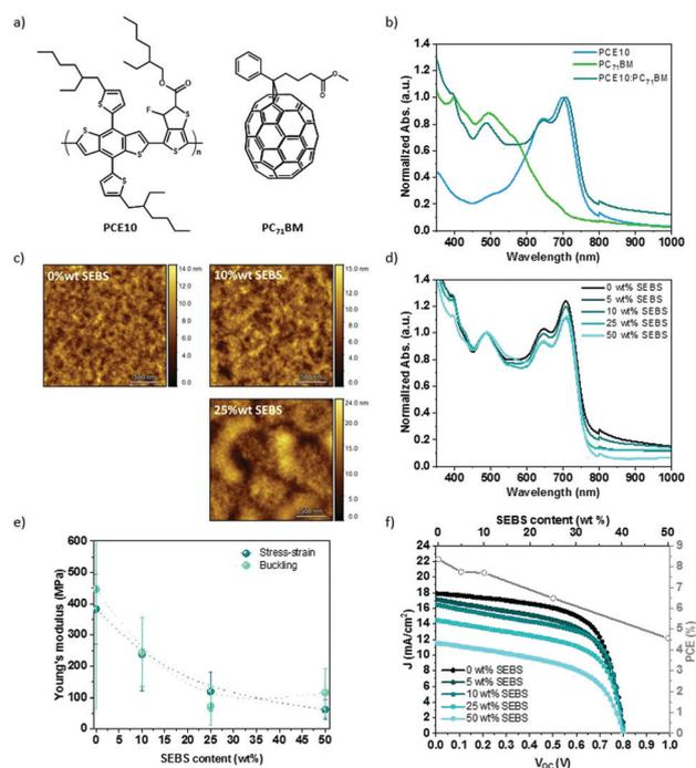
Fig. 7 PCE10:PC<sub>71</sub>BM (1:1.5) solar cell: (a) chemical structures, and (b) absorption spectra. (c) PCE10:PC<sub>71</sub>BM:SEBS morphology characterized by atomic force microscopy. (d) Absorption spectra of PCE10:PC<sub>71</sub>BM film mixed with SEBS elastomer. (e) Young's moduli by stress-strain or buckling methods with different amounts of SEBS (wt/wt% PC<sub>71</sub>BM). (f)  $J$ - $V$  characteristics curves of PCE10:PC<sub>71</sub>BM with SEBS elastomer and associated PCE.
