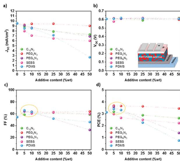
**Fig. 6** Photovoltaic performances of P3HT:PC<sub>61</sub>BM-based OPV in the function of the additive content.
