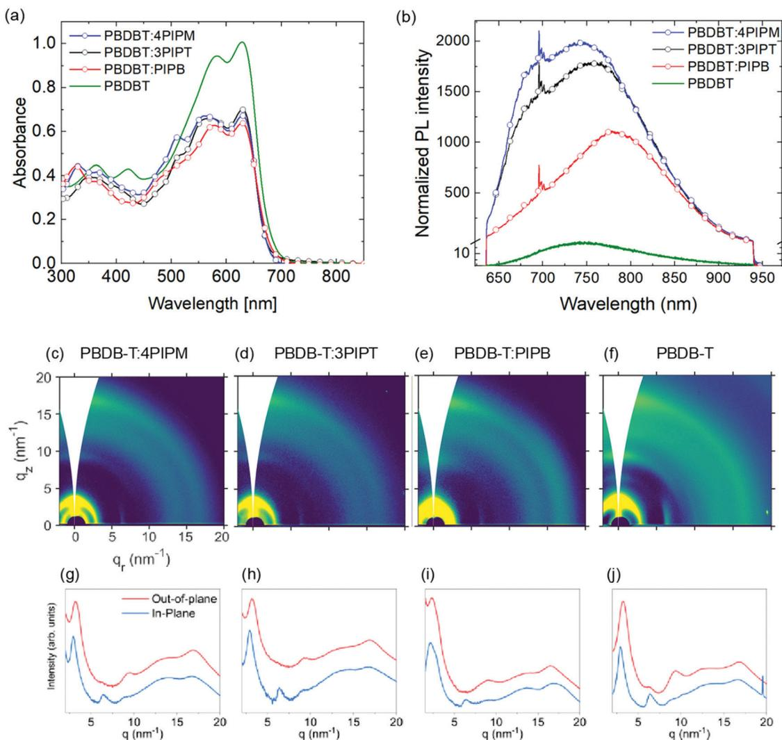
Fig. 6 Solid state (a) UV-vis absorption normalized by the film thickness and (b) photoluminescence spectra normalized by the absorption at 633 nm for **PBDBT:PIPB** (red), **PBDBT:3PIPT** (black), **PBDBT:4PIPM** (blue) and **PBDBT** (green). 2D GIWAXS patterns and the out-of-plane (OOP) and in-plane (IP) cuts of the corresponding 2D-GIWAXS patterns of **PBDBT:4PIPM** (c and g), **PBDBT:3PIPT** (d and h), **PBDBT:PIPB** (e and i) and **PBDBT** (f and j).
