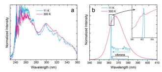
Fig. 3 (a) PLE and PL spectra of  $SrB_4O_7$ : $Eu^{2+}$  microparticles. The PLE spectrum was monitored at 367.2 nm and recorded at 11 and 300 K. (b) PL spectra recorded at 11 K and 300 K excited at 300 nm. In-depth analysis of the ZPL lines and vibronic transitions was presented in ref. 8.
