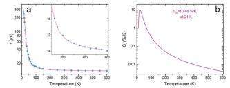
Fig. 5 (a) Average decay time  $\bar{\tau}$  (eqn (3)) of SrB<sub>4</sub>O<sub>7</sub>:Eu<sup>2+</sup> under 300 nm excitation and monitored at 362.4 nm. (b) Calculated relative thermal sensitivity of the investigated phosphor
