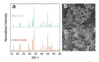
Fig. 2 (a) X-Ray diffraction pattern of  $SrB_4O_7$  containing 3% of  $Eu^{2+}$  and prepared in an air atmosphere. (b and c) SEM images of the  $SrB_4O_7$ : $Eu^{2+}$  powder, taken at different magnifications (b - 5  $\mu$ m scale bar; c - 2  $\mu$ m scale bar).
